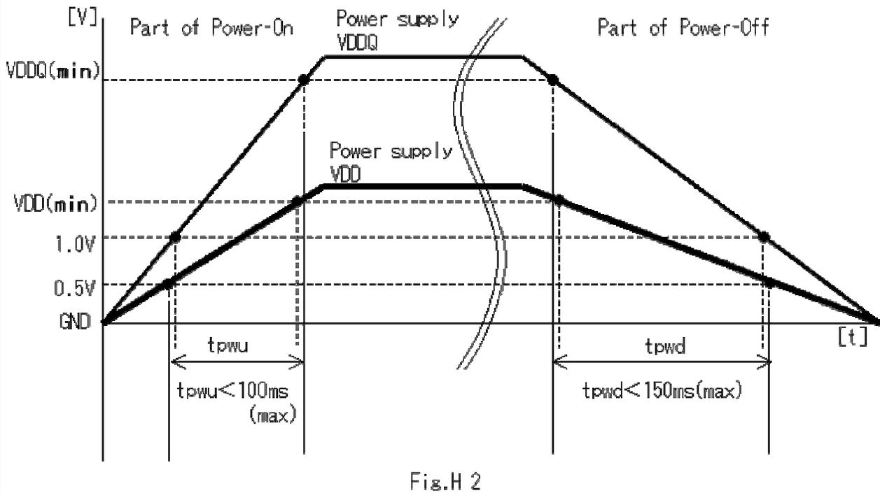
Fig.H Power-On and Power-Off procedure
