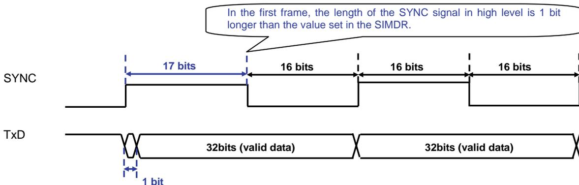
(Example): With the SIOF Master Mode 2, Frame Length = 32 bits
