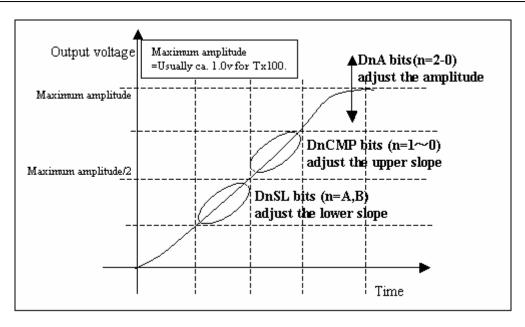
Figure. The roles of corresponding bits. (ex. for rising waveform)
