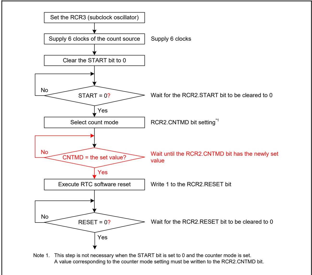
Figure 26.3 Clock and Count Mode Setting Procedure
