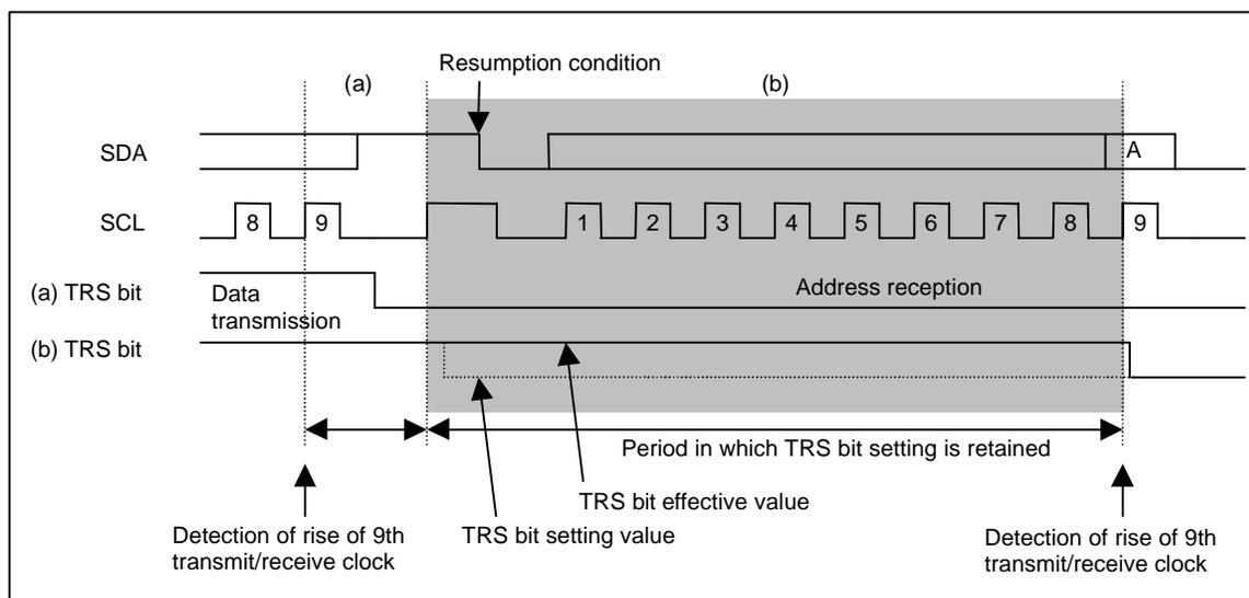
**Figure 2 Scheme of TRS Bit Setting in Slave Mode**
