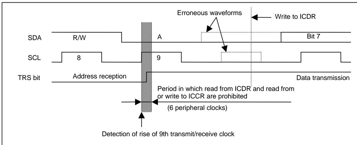
**Figure 1 Scheme of Slave Transmit Operation**
