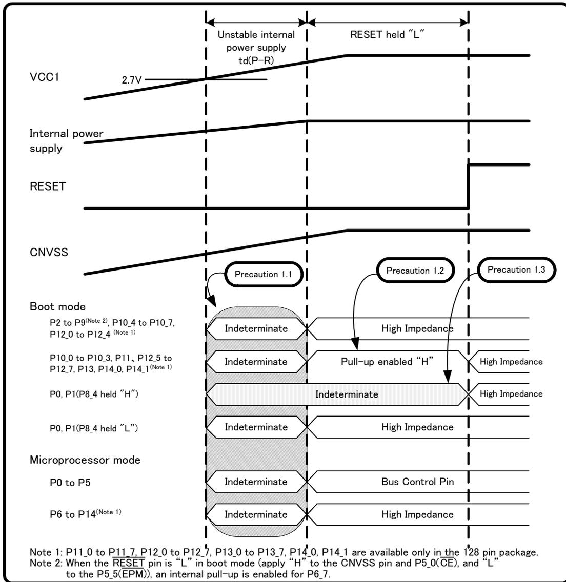
Figure 1. Pin State when Power is Turned On in Boot Mode and Microprocessor Mode
