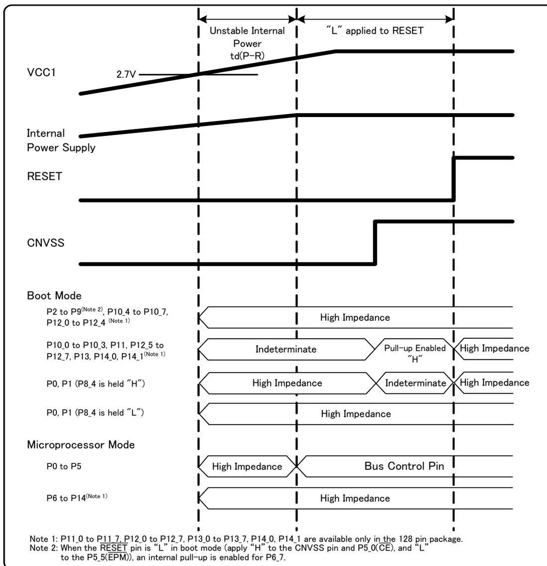
Figure 2. Pin State when Countermeasure is Followed and Power is Turned On
