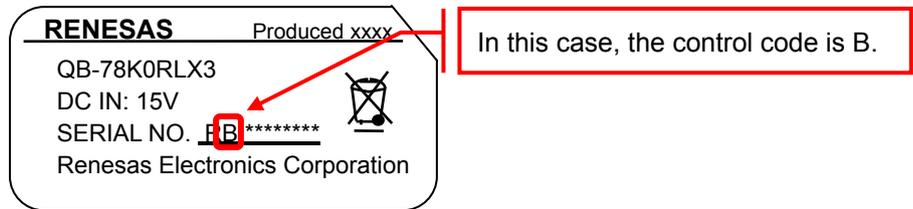
**Figure 2. Checking the Control Code (ID78K0R-QB)**
