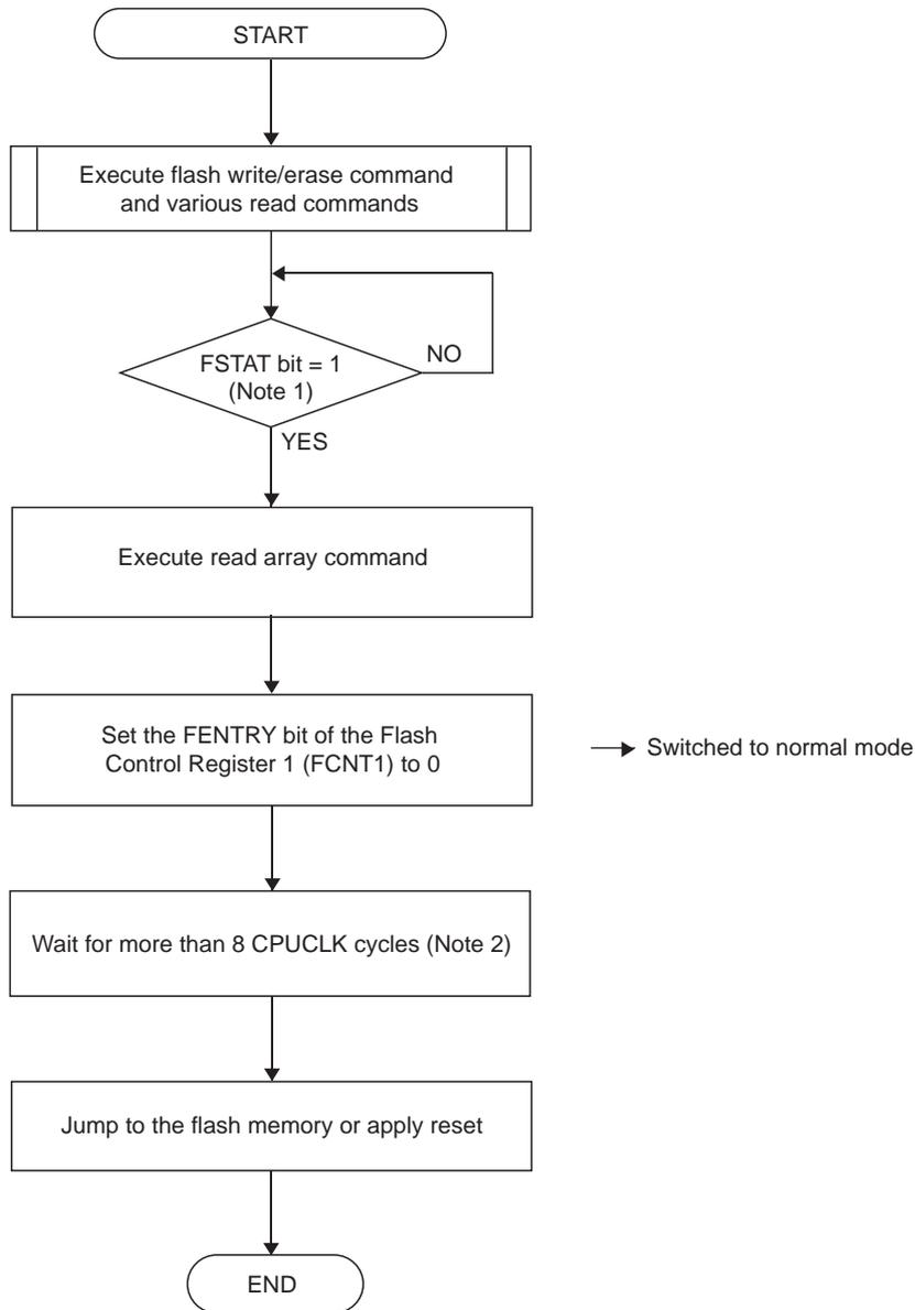
Note1: If it is checked that the value of FSTAT bit in Flash Status Register 1 (FSTAT1) is "1" after executing the command in flash E/W enable mode, it is not necessary to check that the value of FSTAT bit is "1".
