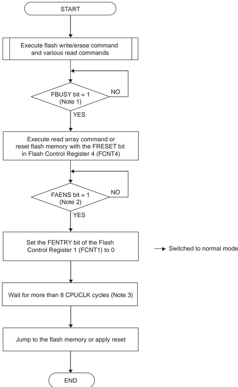
Note1: If it is checked that the value of FBUSY bit in Flash Status Register (FSTAT) is "1" after executing the command in flash E/W enable mode, it is not necessary to check that the value of FBUSY bit is "1".
