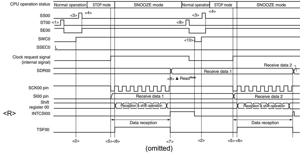
Figure 12-72. Timing Chart of SNOOZE Mode Operation (Continuous Startup) (Type 1: DAPmn = 0, CKPmn = 0)
