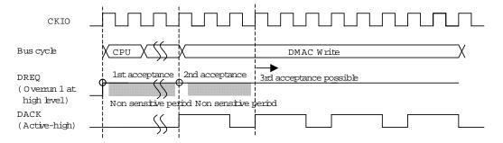
Fig3. Example of DREQ Input Detection in Cycle StealMode LevelDetection When DACK is split to 4 due to Idle Cycles.
