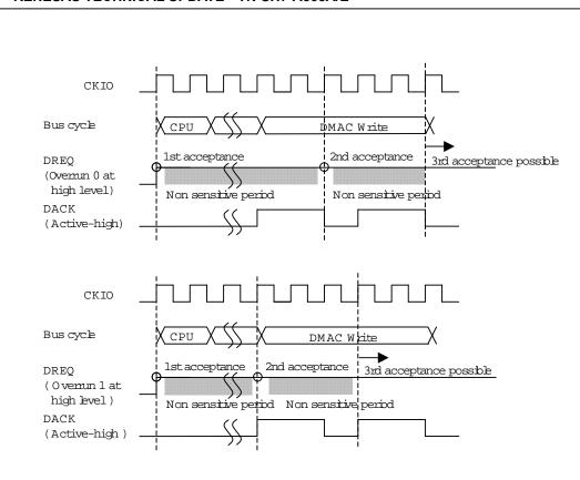
Fig4.Example of DREQ Input Detection in Cycle StealMode LevelDetection When DACK is split to 2 due to Idle Cycles.
