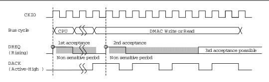
Figl.Example of DREQ Input Detection in Cycle StealMode Edge Detection When DACK is split to 4 due to Idle Cycles.
