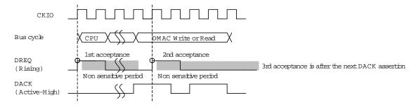
Fig2 Example of DREQ Input Detection in Cycle StealMode Edge Detection When DACK is split to 2 due to Idle Cycles.
