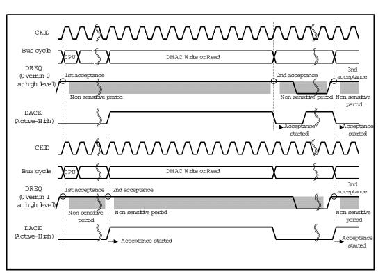
Fig4. Example of DREQ Input Detection in Cycle Steal Mode Level Detection When DACK is not split to 4 due to Idle Cycles. (Correction)
