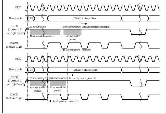
Fig3. Example of DREQ Input Detection in Cycle Steal Mode Level Detection
