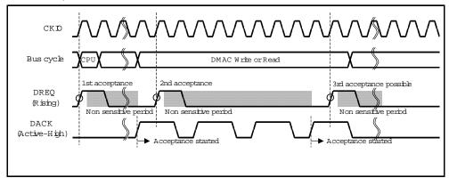
$\label{eq:Fig1.example} \textit{Fig1. Example of DREQ Input Detection in Cycle Steal Mode Edge Detection}$
