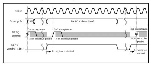
Fig2. Example of DREQ Input Detection in Cycle Steal Mode Edge Detection
