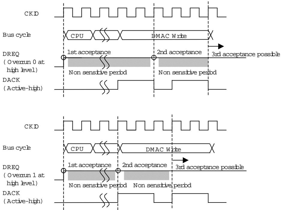
Fig4. Example of DREQ Input Detection in Cycle Steal Mode Level Detection When DACK is split to 2 due to Idle Cycles.
