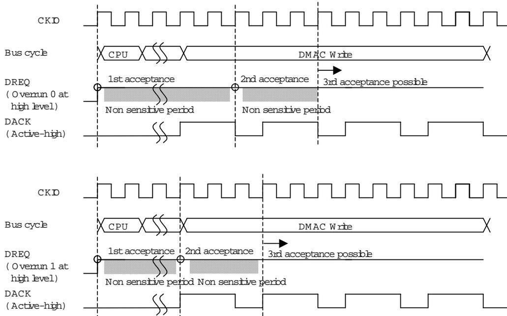
Fig3. Example of DREQ Input Detection in Cycle Steal Mode Level Detection
