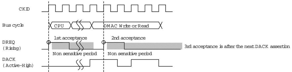
Fig2 Example of DREQ Input Detection in Cycle Steal Mode Edge Detection
