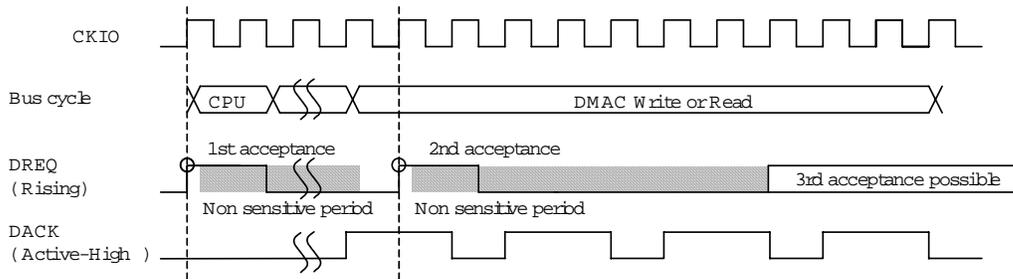
Fig1.Example ofDREQ Input Detection in Cycle Steal Mode Edge Detection
