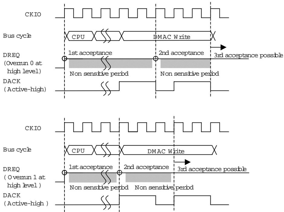
Fig4. Example of DREQ Input Detection in Cycle Steal Mode Level Detection
