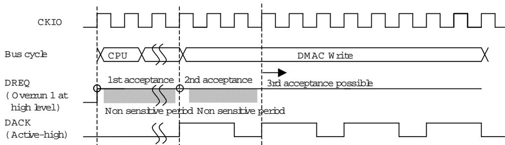
Fig3.Example ofDREQ Input Detection in Cycle Steal Mode Level Detection
