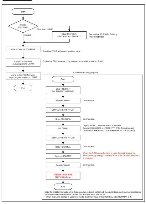
Procedure for Firmware Transfer to FCU RAM 1
