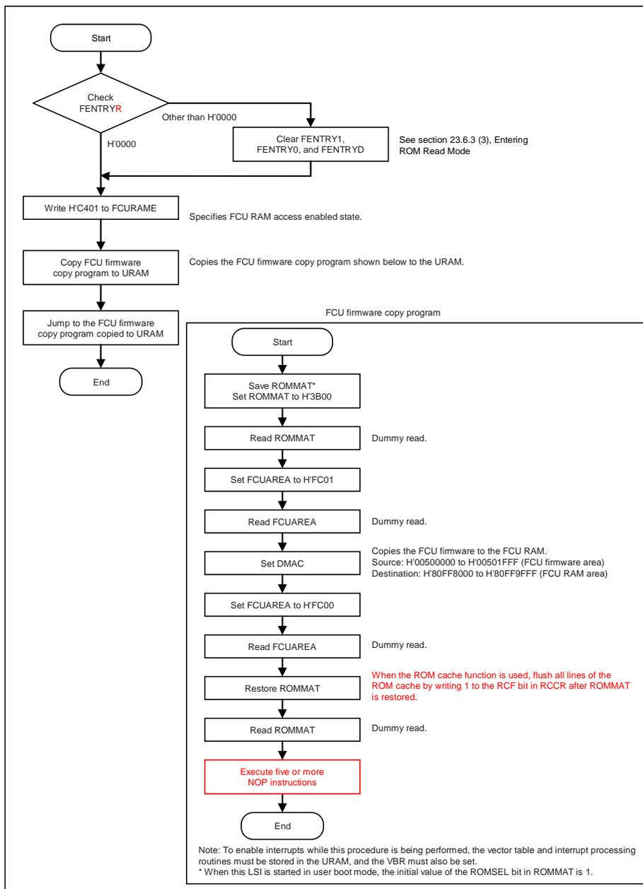
Procedure for Firmware Transfer to FCU RAM 1
