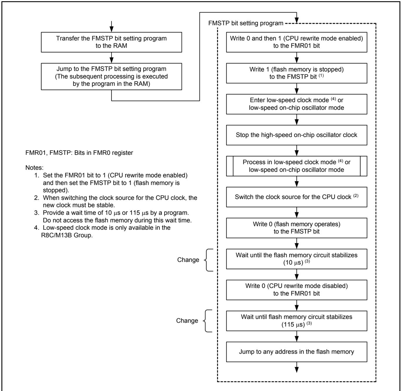
Figure 3. Procedure for Reducing Power Consumption Using the FMSTP Bit
