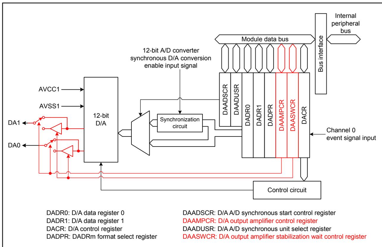
**Figure 51.1 Block Diagram of 12-Bit D/A Converter**
