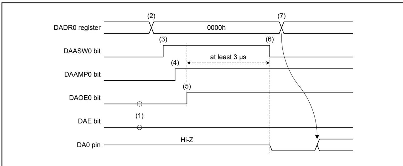
Figure 51.4 Initial Setting Procedure of the Output Buffer Amplifier
