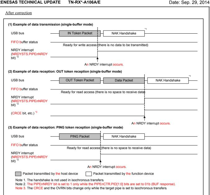
Figure 25.9 Timing of NRDY Interrupt Generation (When Function Controller Function is Selected)
