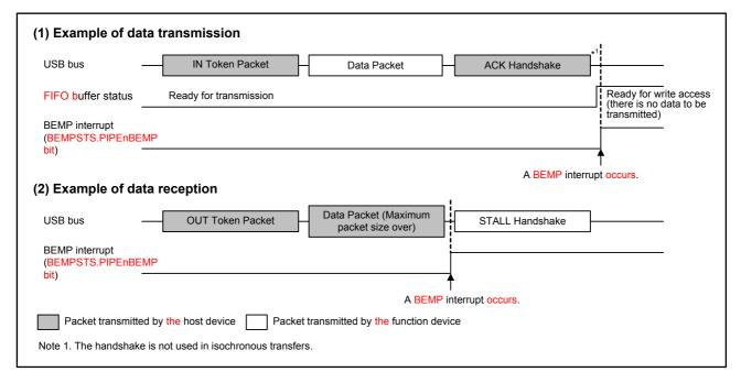
Figure 25.10 Timing of BEMP Interrupt Generation (When Function Controller Function is Selected)
