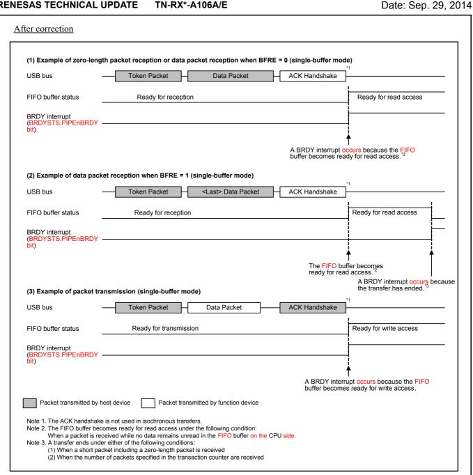
Figure 25.8 Timing of BRDY Interrupt Generation
