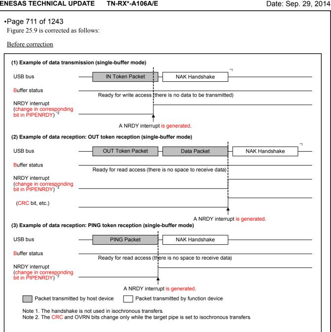
Figure 25.9 Timing of NRDY Interrupt Generation (When Function Controller is Selected)
