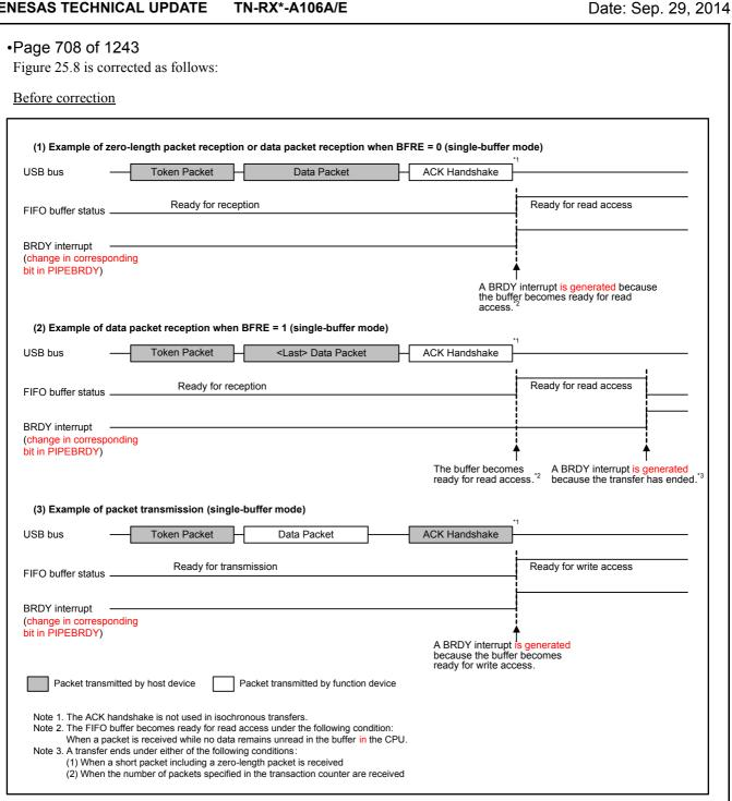
Figure 25.8 Timing of BRDY Interrupt Generation
