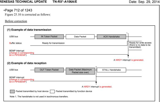
Figure 25.10 Timing of BEMP Interrupt Generation (When Function Controller is Selected)
