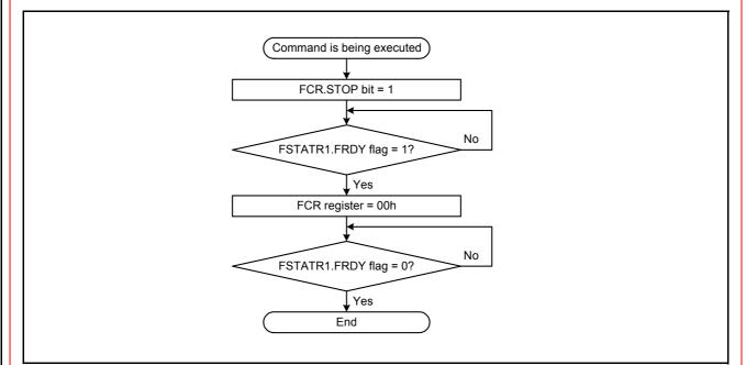
Figure 35.xx Procedure for Forced Stop of Software Commands
