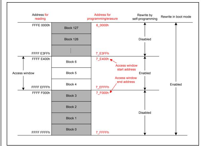
Figure 35.4 Area Protection Overview (Set Blocks 4 to 6 as the Access Window)
