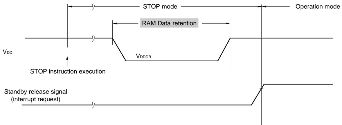
**15. 33.7 Data Memory STOP Mode Low Supply Voltage Data Retention Characteristics**
