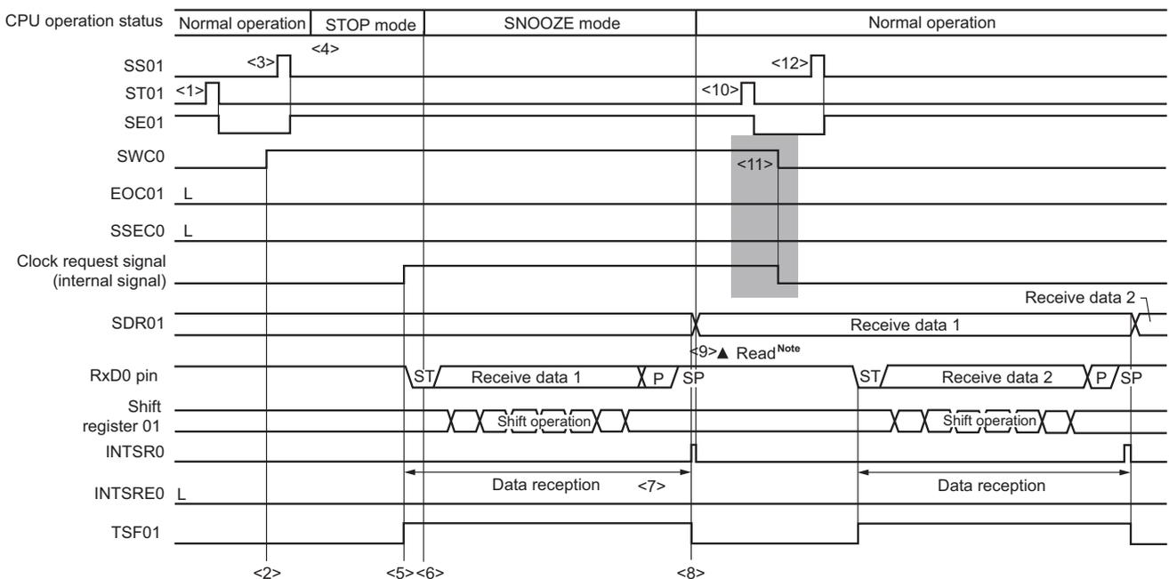
Incorrect the timing chart of clock request signal (internal signal) and SDR01 is revised.
