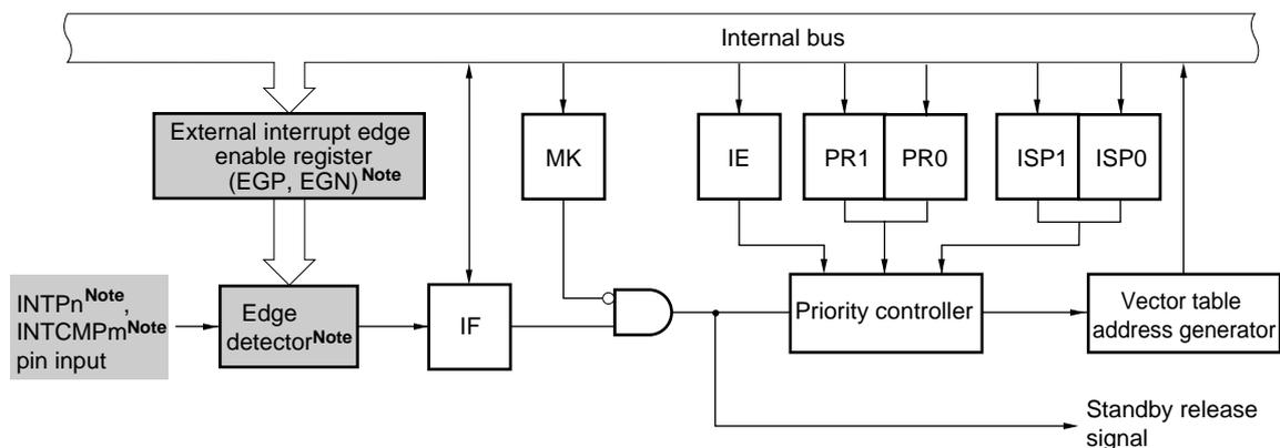
**Note** According to setting for using of the timer KB simultaneous function (the timer KB forced output stop function and timer restart function), the interrupt signal pass and the interrupt generation timing and the edge enable register for INTP20 and INTP21 and INTCMP<sup>m</sup> vary. For details, see **14.5 Caution for Using Timer KB Simultaneous Operation Function.**
