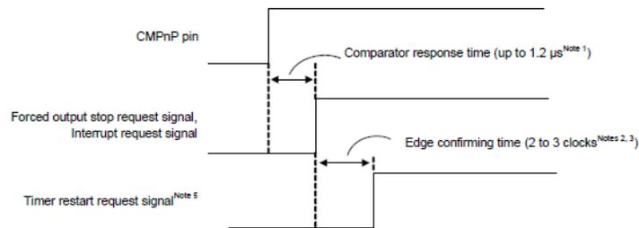
Note 1. When noise filtering is set to “0, 0” by using the CnDFS1 and CnDFS0 bits in the comparator n control register (CnCTL).
