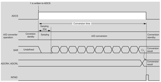
A/D conversion is performed once when the bit 7 (ADCS) of the A/D converter mode register 0 (ADM0) is set to 1 by software. The ADCS bit is automatically cleared to 0 after A/D conversion ends.
