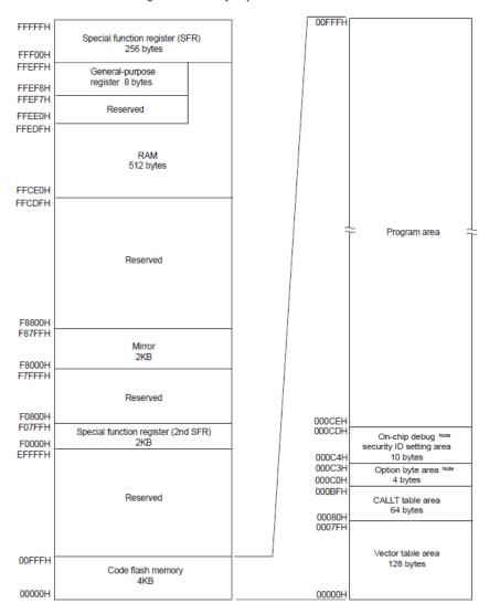
Note Set the option bytes to 000C0H to 000C3H, and the on-chip debug security IDs to 000C4H to 000CDH.
