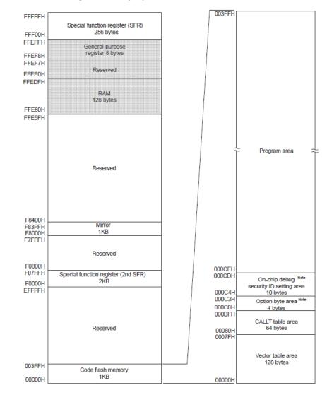
Note Set the option bytes to 000C0H to 000C3H, and the on-chip debug security IDs to 000C4H to 000CDH.
