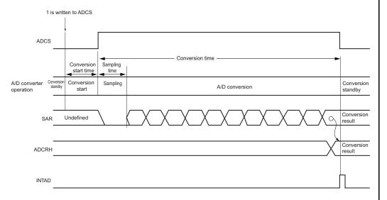
A/D conversion is performed once when the bit 7 (ADCS) of the A/D converter mode register 0 (ADM0) is set to 1 by software.
