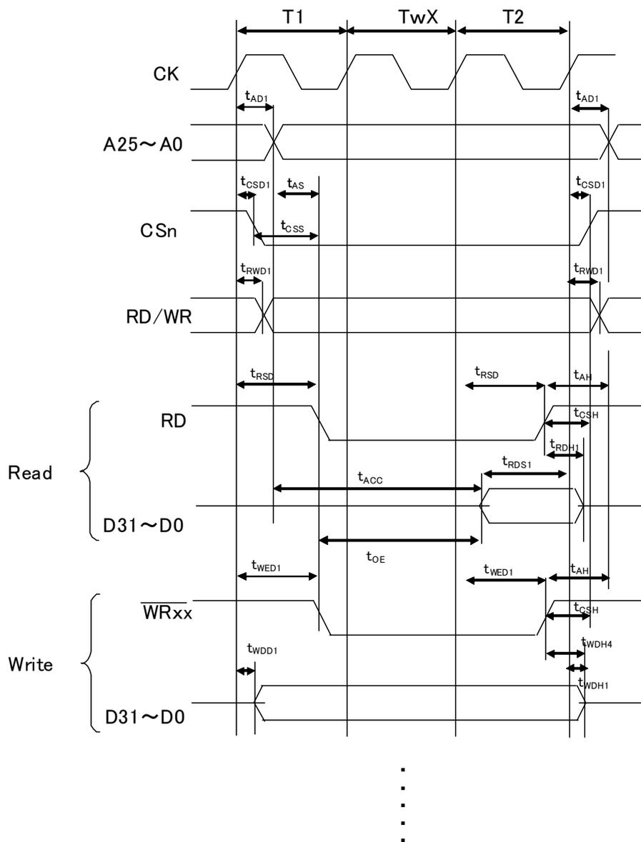
Figure 31.13 Normal Space Basic Bus Cycle (Insertion of External Wait 1)
