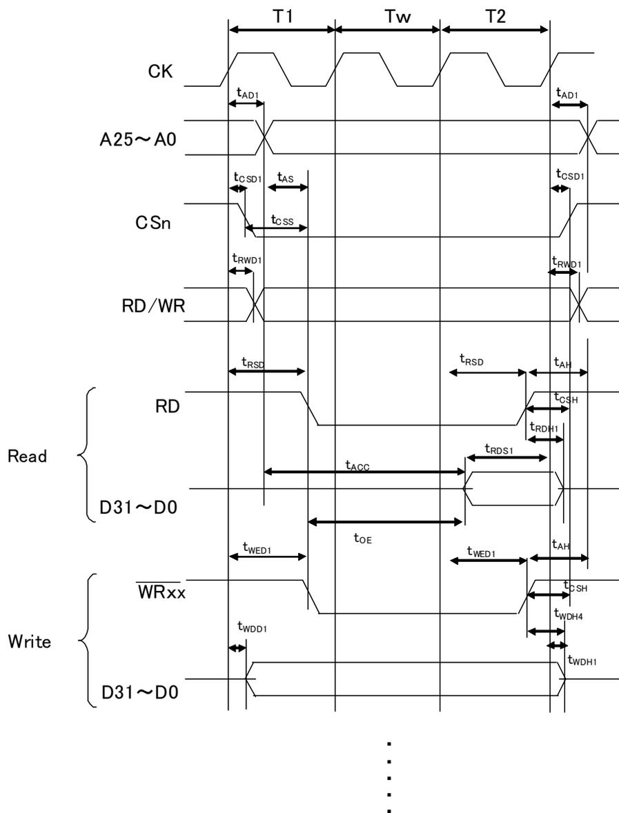
Figure 31.12 Normal Space Basic Bus Cycle (Software Wait 1)
