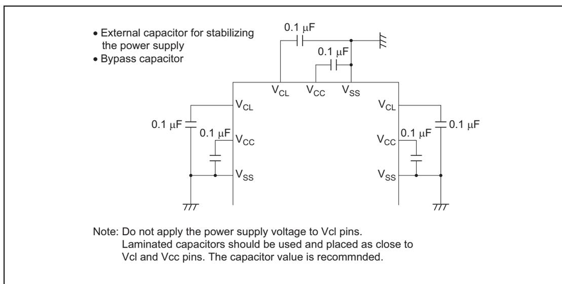
Figure 31.62 Method of Connecting Capacitors
