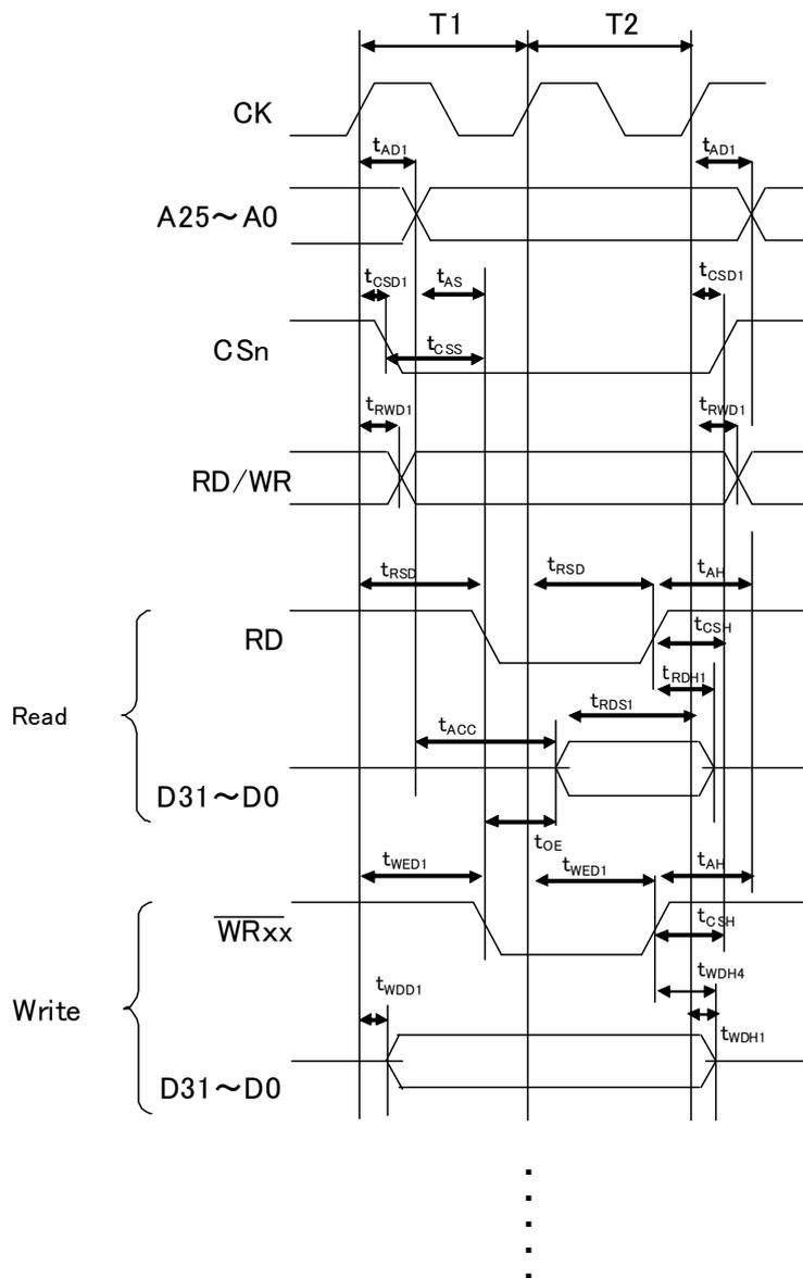
Figure 31.11 Normal Space Basic Bus Cycle (No Wait)
