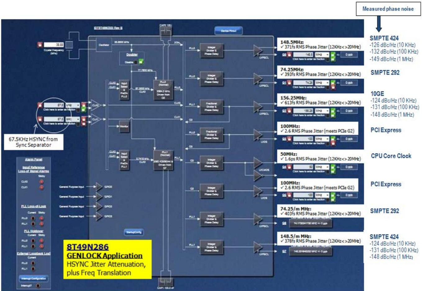
Figure 4b: Corresponding 8T49N287 Timing Commander GUI Configuration
