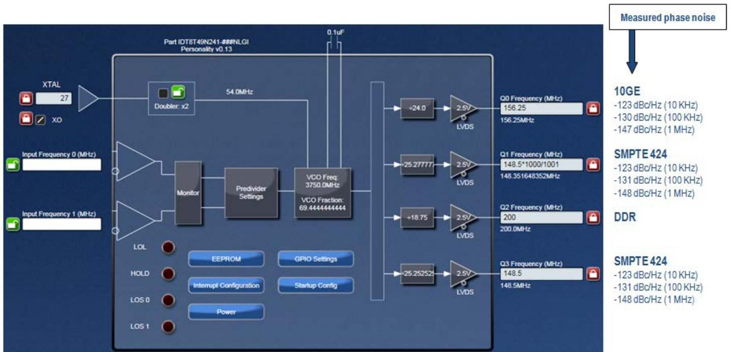
Figure 3a: Corresponding 8T49N241 Timing Commander GUI Configuration
