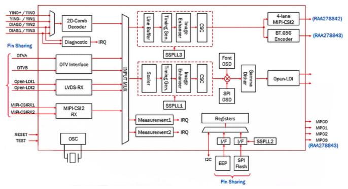
Figure 1. RAA278842, RAA278843 Functional Block Diagram
