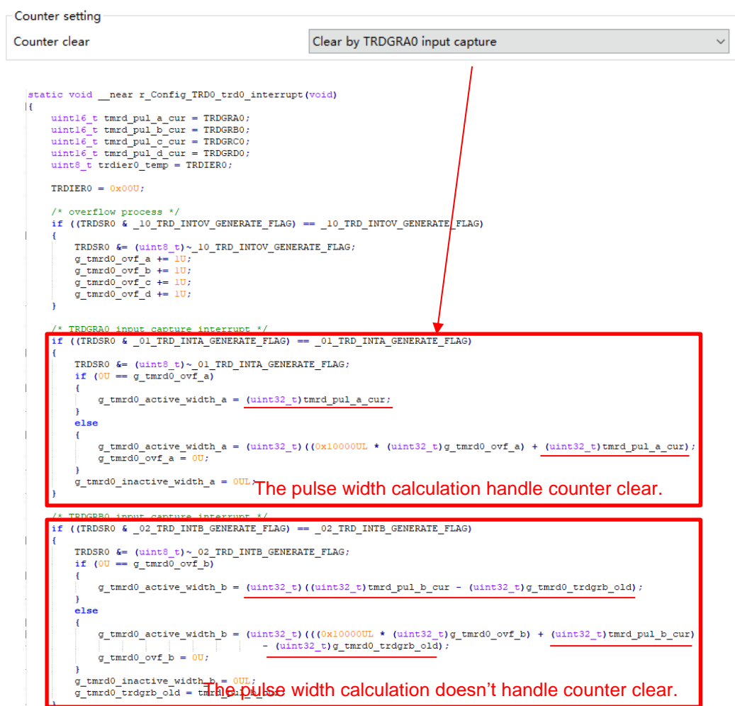
Figure 6-3 Counter clear setting in Input capture function
