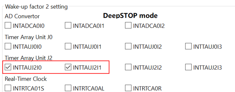
Figure 3-5 Wake-up factor 2 setting in DeepSTOP mode
