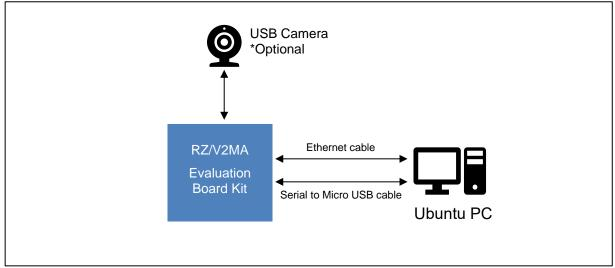
Figure 4-1 Hardware Configuration
