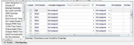
Pin Function List allows user to change a specific pin which has been to set by CG. For example, IRQ7 has been set by CG. an available pin are automatically set.
