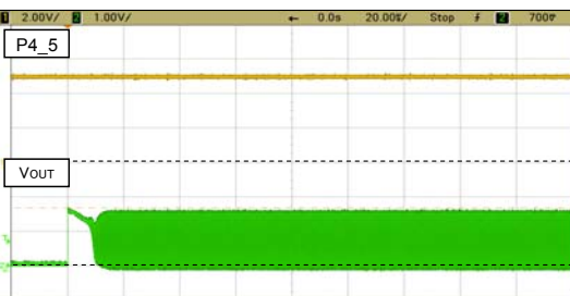
Oscillation start up waveform on recommendable circuit condition MODEL: CSTCE20M0V53-R0 with R5F2138CCDFP(CM11=0)
