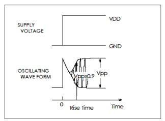
In the case that rising time of Vdd(Vset) is slow comparing to resonator's rise time due to the bypass capacitor, resonator's rise time is also slow because it depends on rising time of Vdd(Vset).
