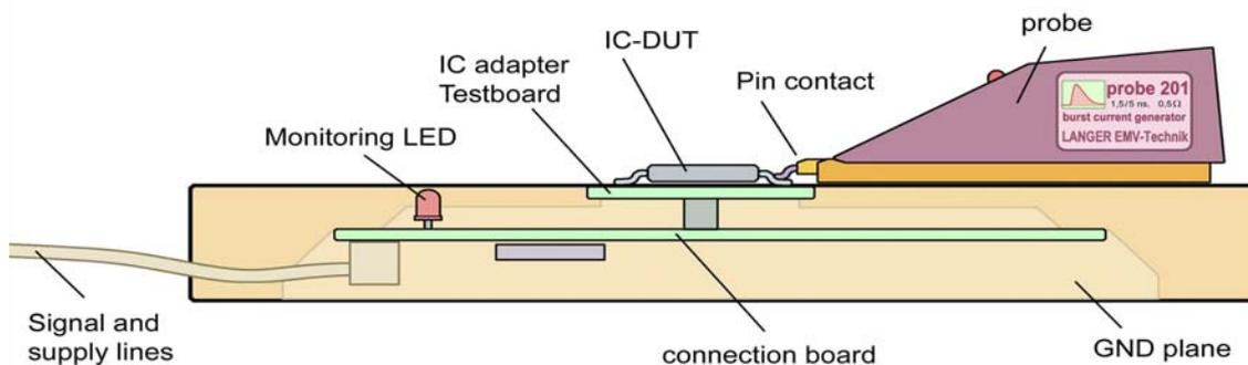
Depending on the kind of measurement, different burst generators (probes) can be used. These probes are placed on the reference plane and are electrically connected to it. A pin contact is used to couple the bursts into the IC pin. This measuring setup, especially the usage of a reference plane, guarantees that correct measurements up to the GHz range can be performed.
