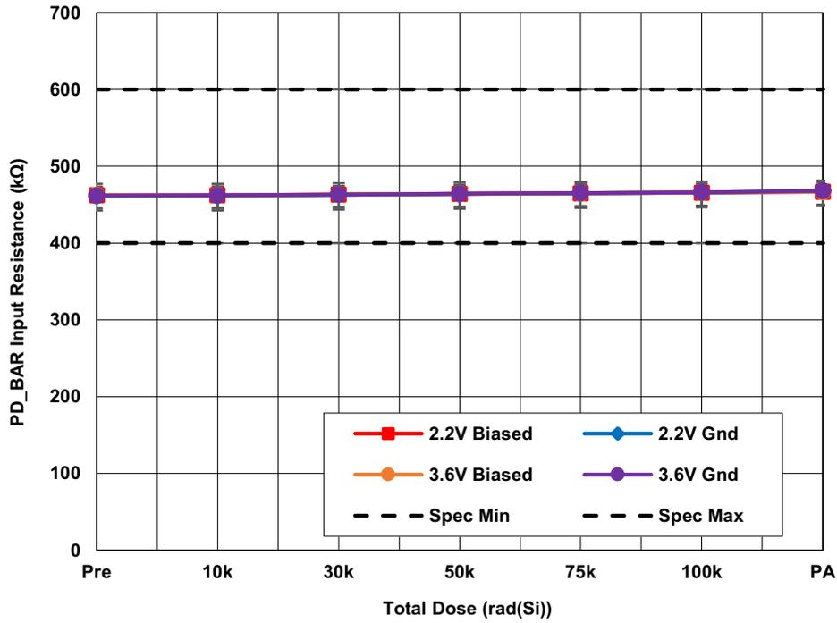
Figure 26. ISL73141SEHMFN average  $\overline{R_{INPDL}}$  with  $AV_{CC} = 3.3V$ ,  $DV_{CC} = 3.6V$  and  $2.2V$  and  $REF = 3.0V$  as a function of LDR irradiation and anneal. The error bars represent the minimum and maximum measured values. The datasheet limits are  $400k\Omega$  minimum and  $600k\Omega$  maximum.
