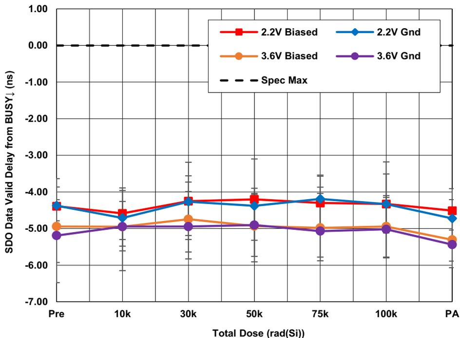
Figure 29. ISL73141SEHMFN average SDO data valid delay from BUSY falling edge ( $t_{DBUSY_{LSDOV}}$ ) with  $AV_{CC} = 3.0V$ ,  $DV_{CC} = 2.2V$  and  $AV_{CC} = 3.6V$ ,  $DV_{CC} = 3.6V$ ,  $REF = 3.0V$ ,  $f_{SAMP} = 750kps$ ,  $A_{IN} = -1dbFS$  and  $C_L = 10pF$  as a function of LDR irradiation and anneal. The error bars represent the minimum and maximum measured values. The datasheet limit is 0ns maximum.
