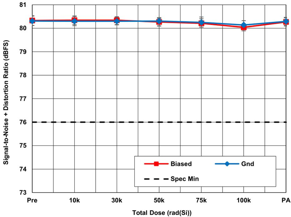
Figure 9. ISL73141SEHMFN average signal to noise + distortion ratio (SINAD) with  $AV_{CC} = 3.3V$ ,  $DV_{CC} = 2.5V$ ,  $REF = 3.0V$ ,  $f_{SAMP} = 105ksps$ , and  $A_{IN} = -1dBFS$  as a function of LDR irradiation and anneal. The error bars represent the minimum and maximum measured values. The datasheet limit is 76dB minimum.
