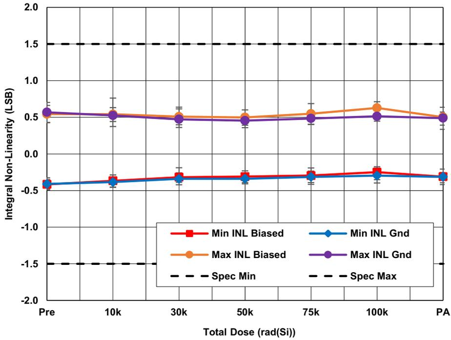
Figure 4. ISL73141SEHMFN average minimum and maximum integral non-linearity (INL) with  $AV_{CC} = 3.3V$ ,  $DV_{CC} = 2.5V$ ,  $REF = 3.0V$ ,  $f_{SAMP} = 750kpsps$ , and  $A_{IN} =$  full-scale sine wave as a function of LDR irradiation and anneal. The error bars represent the minimum and maximum measured values. The datasheet limits are -1.5 LSB minimum and 1.5 LSB maximum.
