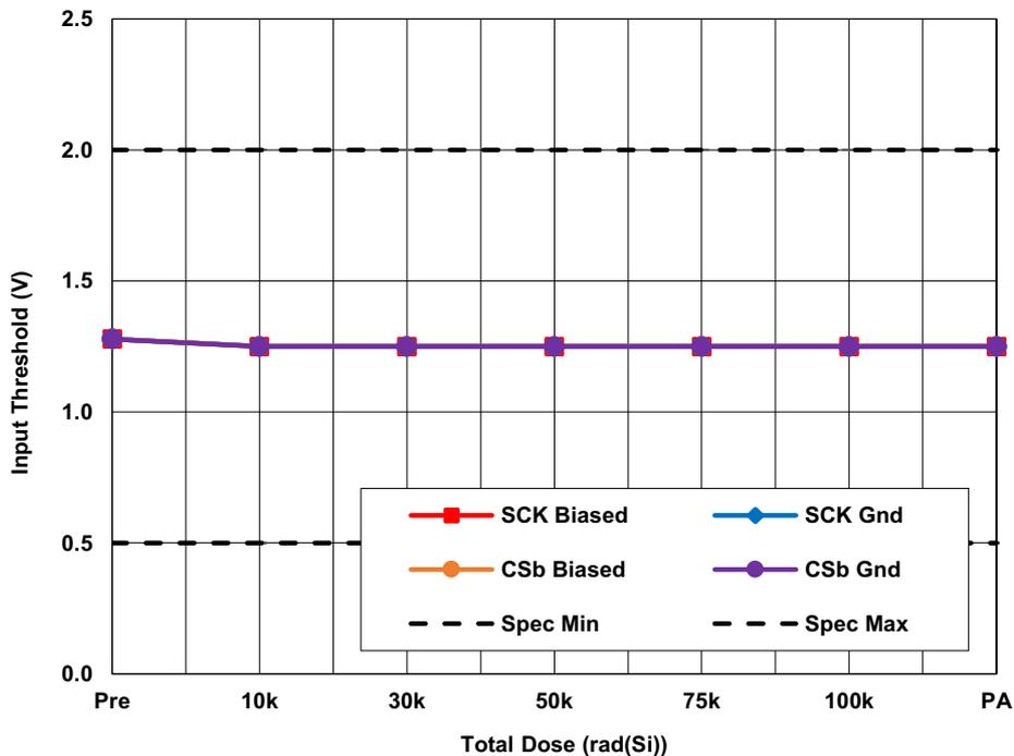
Figure 21. ISL73141SEHMFN average high level input ( $V_{IH}$ ) and low level input ( $V_{IL}$ ) with  $AV_{CC} = 3.3V$ ,  $DV_{CC} = 2.5V$  and  $REF = 3.0V$  as a function of LDR irradiation and anneal. The error bars (if visible) represent the minimum and maximum measured values. The datasheet limit for  $V_{IH}$  is 2.0V minimum and the datasheet limit for  $V_{IL}$  is 0.5V maximum.
