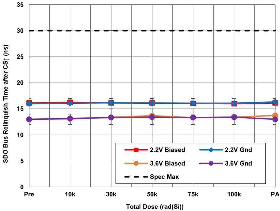
Figure 32. ISL73141SEHMFN average SDO bus relinquish time after  $\overline{CS}$  rising edge ( $t_{DCSHSDOZ}$ ) with  $AV_{CC} = 3.0V$ ,  $DV_{CC} = 2.2V$  and  $AV_{CC} = 3.6V$ ,  $DV_{CC} = 3.6V$ ,  $REF = 3.0V$ ,  $f_{SAMP} = 750ksps$ ,  $A_{IN} = -1dbFS$  and  $C_L = 10pF$  as a function of LDR irradiation and anneal. The error bars represent the minimum and maximum measured values. The datasheet limit is 30ns maximum.
