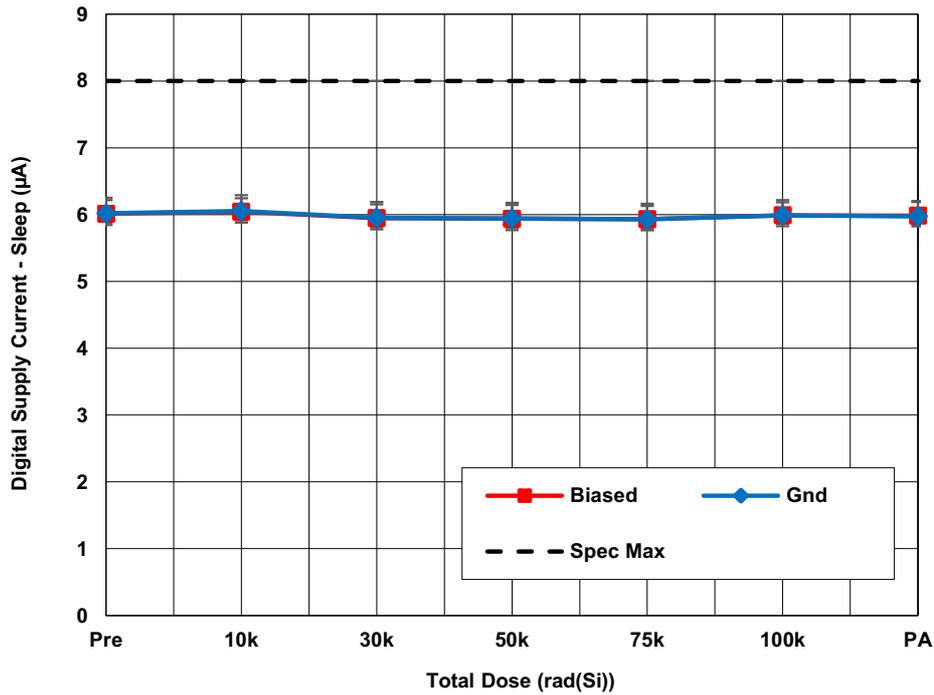
Figure 20. ISL73141SEHMFN average digital supply current - sleep ( $I_{SLDVCC}$ ) with  $AV_{CC} = 3.3V$ ,  $DV_{CC} = 2.5V$ ,  $REF = 3.0V$ ,  $PD = GND$  as a function of LDR irradiation and anneal. The error bars represent the minimum and maximum measured values. The datasheet limit is 8µA maximum.
