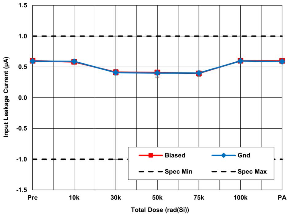
Figure 13. ISL73141SEHMFN average input leakage current ( $I_{A_{IN}}$ ) with  $AV_{CC} = 3.3V$ ,  $DV_{CC} = 2.5V$  and  $REF = 3.0V$  as a function of LDR irradiation and anneal. The error bars represent the minimum and maximum measured values. The datasheets limits are  $-1\mu A$  minimum and  $1\mu A$  maximum.
