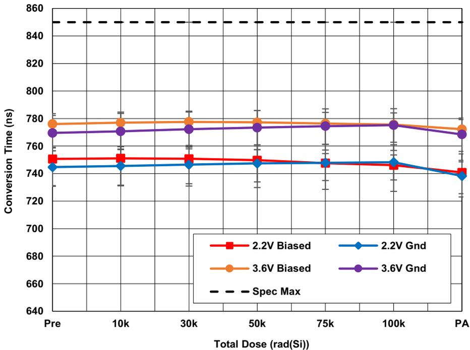
Figure 27. ISL73141SEHMFN average conversion time ( $t_{CONV}$ ) with  $AV_{CC} = 3.0V$ ,  $DV_{CC} = 2.2V$  and  $AV_{CC} = 3.6V$ ,  $DV_{CC} = 3.6V$ ,  $REF = 3.0V$ ,  $f_{SAMP} = 750ksps$  and  $A_{IN} = -1dbFS$  as a function of LDR irradiation and anneal. The error bars represent the minimum and maximum measured values. The datasheet limit is  $850ns$  maximum.
