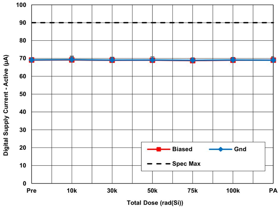
Figure 18. ISL73141SEHMFN average digital supply current - active ( $I_{DVCC}$ ) with  $AV_{CC} = 3.3V$ ,  $DV_{CC} = 2.5V$ ,  $REF = 3.0V$ ,  $f_{SCK} = 33MHz$ , and  $C_L = 10pF$  as a function of LDR irradiation and anneal. The error bars represent the minimum and maximum measured values. The datasheet limit is  $90\mu A$  maximum.
