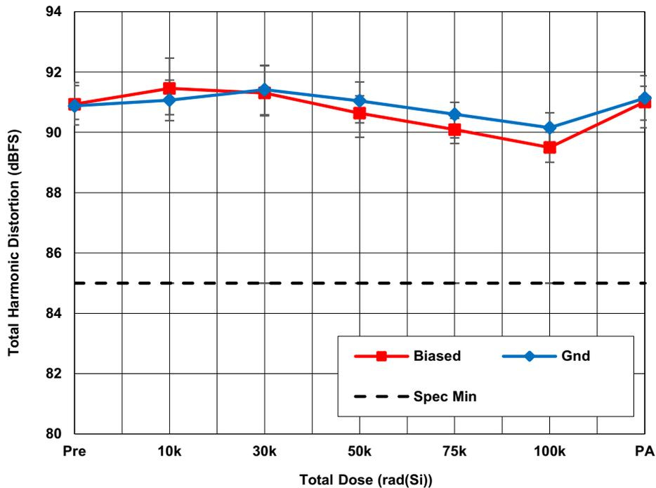
Figure 11. ISL73141SEHMFN average total harmonic distortion (THD) with  $AV_{CC} = 3.3V$ ,  $DV_{CC} = 2.5V$ ,  $REF = 3.0V$ ,  $f_{SAMP} = 105ksps$  (first five harmonics), and  $A_{IN} = -1dBFS$  as a function of LDR irradiation and anneal. The error bars represent the minimum and maximum measured values. The datasheet limit is 85db minimum.
