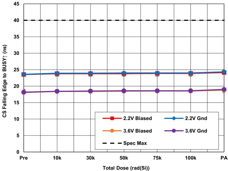
Figure 28. ISL73141SEHMFN average  $\overline{CS}$  falling edge to BUSY rising edge ( $t_{BUSY_{LH}}$ ) with  $AV_{CC} = 3.0V$ ,  $DV_{CC} = 2.2V$  and  $AV_{CC} = 3.6V$ ,  $DV_{CC} = 3.6V$ ,  $REF = 3.0V$ ,  $f_{SAMP} = 750kps$ ,  $A_{IN} = -1dbFS$  and  $C_L = 10pF$  as a function of LDR irradiation and anneal. The error bars represent the minimum and maximum measured values. The datasheet limit is 40ns maximum.
