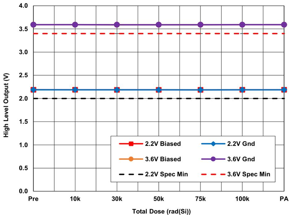
Figure 23. ISL73141SEHMFN average high-level output ( $V_{OH}$ ) with  $AV_{CC} = 3.3V$ ,  $DV_{CC} = 3.6V$  and  $2.2V$ ,  $REF = 3.0V$  and  $I_O = -500\mu A$  as a function of LDR irradiation and anneal. The error bars (if visible) represent the minimum and maximum measured values. The datasheet limits are  $2.0V$  minimum for  $DV_{CC} = 2.2V$  and  $3.4V$  minimum for  $DV_{CC} = 3.6V$ .
