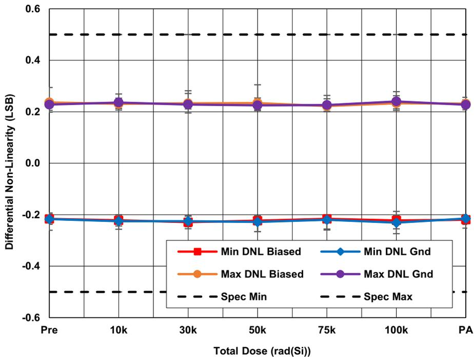
Figure 5. ISL73141SEHMFN average minimum and maximum differential non-linearity (DNL) with  $AV_{CC} = 3.3V$ ,  $DV_{CC} = 2.5V$ ,  $REF = 3.0V$ ,  $f_{SAMP} = 750kpsps$ , and  $A_{IN} =$  full-scale sine wave as a function of LDR irradiation and anneal. The error bars represent the minimum and maximum measured values. The datasheet limits are -0.5 LSB minimum and 0.5 LSB maximum.
