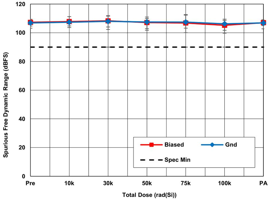
Figure 12. ISL73141SEHMFN average spurious free dynamic range (SFDR) with  $AV_{CC} = 3.3V$ ,  $DV_{CC} = 2.5V$ ,  $REF = 3.0V$ ,  $f_{SAMP} = 105ksps$  (first five harmonics), and  $A_{IN} = -1dBFS$  as a function of LDR irradiation and anneal. The error bars represent the minimum and maximum measured values. The datasheet limit is 90dB minimum.
