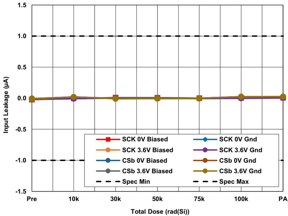
Figure 22. ISL73141SEHMFN average input leakage current ( $I_{IN}$ ) on SCK and  $\overline{CS}$  with  $AV_{CC} = 3.3V$ ,  $DV_{CC} = 2.5V$ ,  $REF = 3.0V$  and  $V_{IN} = 0V$  and  $3.6V$  as a function of LDR irradiation and anneal. The error bars (if visible) represent the minimum and maximum measured values. The datasheet limits are  $-1\mu A$  minimum and  $1\mu A$  maximum.
