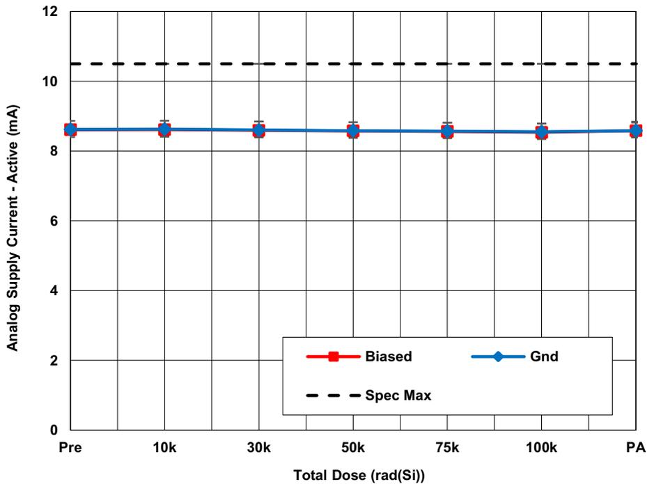
Figure 15. ISL73141SEHMFN average analog supply current - active ( $I_{AVCC}$ ) with  $AV_{CC} = 3.3V$ ,  $DV_{CC} = 2.5V$ ,  $REF = 3.0V$ ,  $f_{SAMP} = 750ksps$ , and  $A_{IN} = -1dBFS$  as a function of LDR irradiation and anneal. The error bars represent the minimum and maximum measured values. The datasheet limit is 10.5mA maximum.
