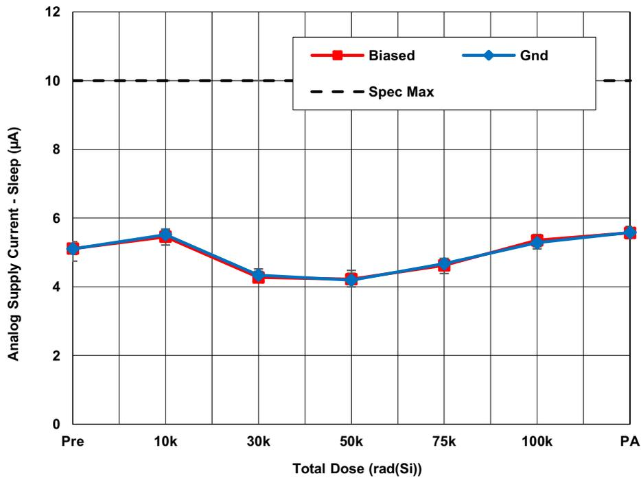
Figure 17. ISL73141SEHMFN average analog supply current - sleep ( $I_{SLAVCC}$ ) with  $AV_{CC} = 3.3V$ ,  $DV_{CC} = 2.5V$ ,  $REF = 3.0V$  and  $PD = GND$  as a function of LDR irradiation and anneal. The error bars represent the minimum and maximum measured values. The datasheet limit is 10µA maximum.
