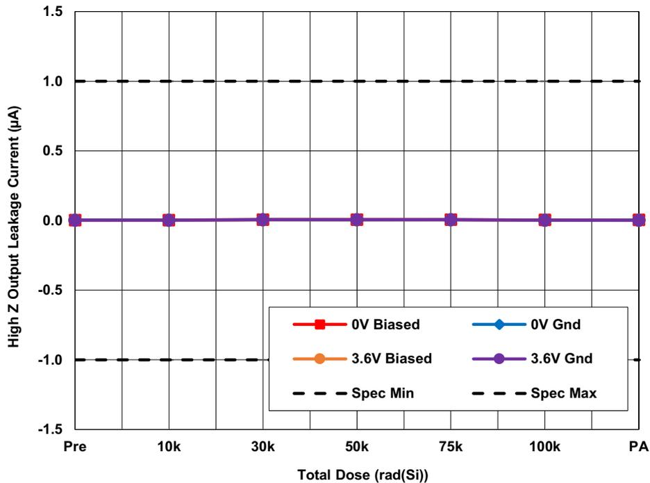
Figure 25. ISL73141SEHMFN average output leakage current ( $I_{OZ}$ ) with  $AV_{CC} = 3.3V$ ,  $DV_{CC} = 3.6V$  and  $0V$  and  $REF = 3.0V$  as a function of LDR irradiation and anneal. The error bars (if visible) represent the minimum and maximum measured values. The datasheet limits are  $-1\mu A$  minimum and  $1\mu A$  maximum.
