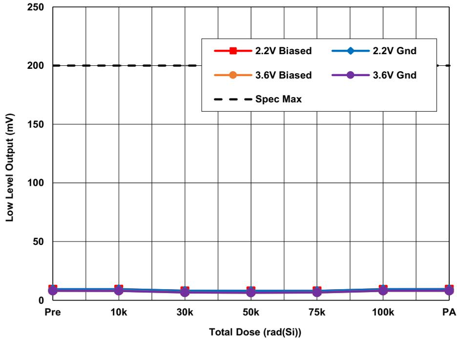
Figure 24. ISL73141SEHMFN average low-level output ( $V_{OL}$ ) with  $AV_{CC} = 3.3V$ ,  $DV_{CC} = 3.6V$  and  $2.2V$ ,  $REF = 3.0V$  and  $I_O = 500\mu A$  as a function of LDR irradiation and anneal. The error bars (if visible) represent the minimum and maximum measured values. The datasheet limit is 200mV maximum.
