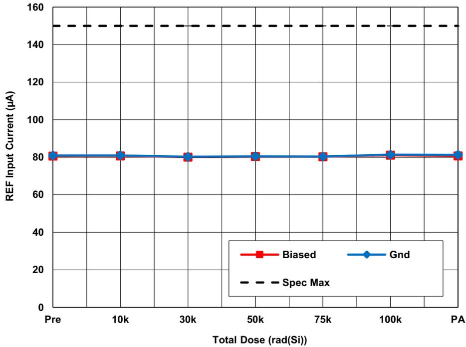
Figure 14. ISL73141SEHMFN average REF input current ( $I_{REF}$ ) with  $AV_{CC} = 3.3V$ ,  $DV_{CC} = 2.5V$  and  $REF = 3.0V$ ,  $f_{SAMP} = 750ksps$  and  $A_{IN} = -1dBFS$  as a function of LDR irradiation and anneal. The error bars represent the minimum and maximum measured values. The datasheet limit is 150µA maximum.
