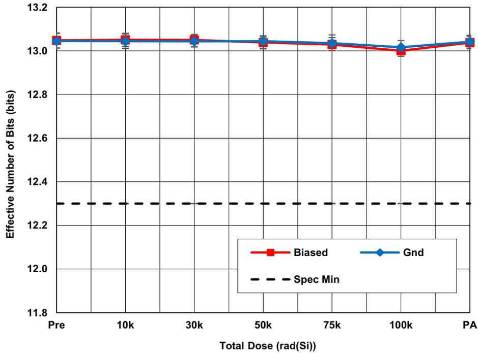
Figure 10. ISL73141SEHMFN average effective number of bits (ENOB) with  $AV_{CC} = 3.3V$ ,  $DV_{CC} = 2.5V$ ,  $REF = 3.0V$ ,  $f_{SAMP} = 105ksps$ , and  $A_{IN} = -1dBFS$  as a function of LDR irradiation and anneal. The error bars represent the minimum and maximum measured values. The datasheet limit is 12.3 bits minimum.
