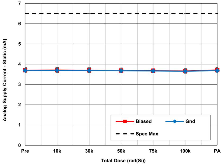
Figure 16. ISL73141SEHMFN average analog supply current - static ( $I_{STATIC}$ ) with  $AV_{CC} = 3.3V$ ,  $DV_{CC} = 2.5V$ ,  $REF = 3.0V$  and  $CS = DV_{CC}$  as a function of LDR irradiation and anneal. The error bars represent the minimum and maximum measured values. The datasheet limit is 6.5mA maximum.
