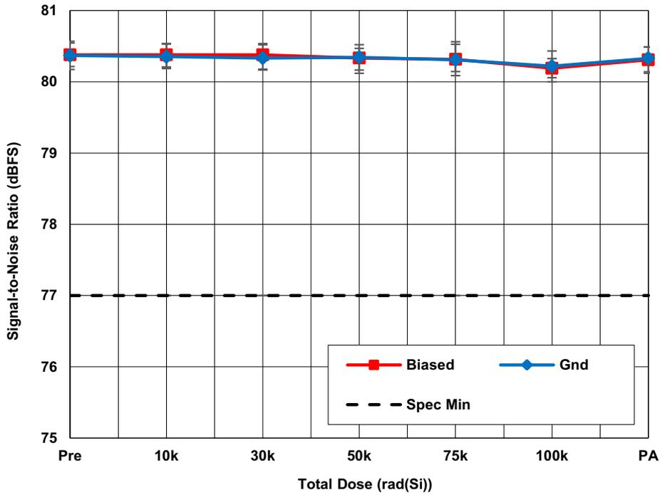
Figure 8. ISL73141SEHMFN average signal to noise ratio (SNR) with  $AV_{CC} = 3.3V$ ,  $DV_{CC} = 2.5V$ ,  $REF = 3.0V$ ,  $f_{SAMP} = 105ksps$ , and  $A_{IN} = -1dBFS$  as a function of LDR irradiation and anneal. The error bars represent the minimum and maximum measured values. The datasheet limit is 77dB minimum.
