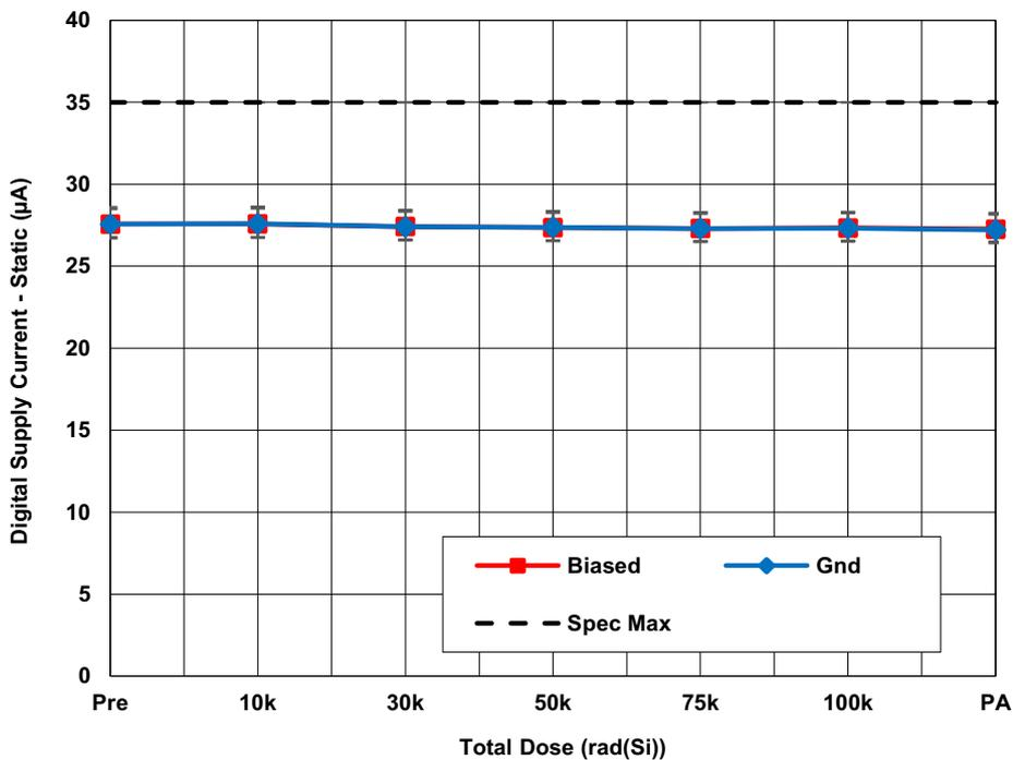
Figure 19. ISL73141SEHMFN average digital supply current - static ( $I_{STDVCC}$ ) with  $AV_{CC} = 3.3V$ ,  $DV_{CC} = 2.5V$ ,  $REF = 3.0V$ ,  $CS = DV_{CC}$  as a function of LDR irradiation and anneal. The error bars represent the minimum and maximum measured values. The datasheet limit is  $35\mu A$  maximum.
