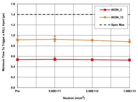
Figure 18. ISL70321SEH minimum time to trigger a KILL input ( $t_{KON}$ ) at  $V_{DD}$  = 3V and 13.2V following irradiation to each level. The error bars (if visible) represent the minimum and maximum measured values. The SMD limit is 1.4µs maximum.
