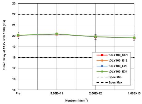
Figure 13. ISL70321SEH timer delay with  $100k\Omega$  resistor ( $t_{DLY_{100}}$ ) at  $V_{DD}$  = 13.2V following irradiation to each level. The error bars (if visible) represent the minimum and maximum measured values. The SMD limits are 18ms minimum and 22ms maximum.
