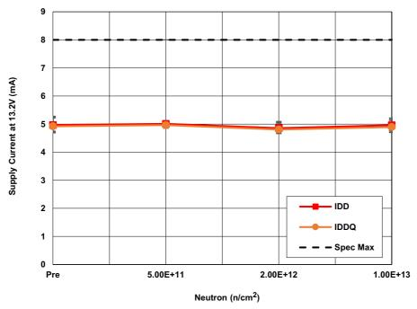
Figure 3. ISL70321SEH quiescent ( $I_{DDQ}$ ) and operating ( $I_{DD}$ ) supply current at  $V_{DD}$  = 13.2V following irradiation to each level. The error bars (if visible) represent the minimum and maximum measured values. The SMD limit is 8mA maximum.
