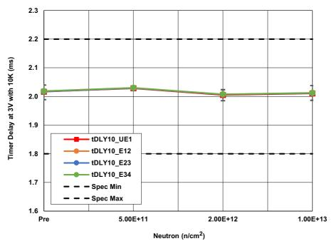
Figure 10. ISL70321SEH timer delay with  $10K\Omega$  resistor ( $t_{DLY_{10}}$ ) at  $V_{DD}$  = 3V following irradiation to each level. The error bars (if visible) represent the minimum and maximum measured values. The SMD limits are 1.8ms minimum and 2.2ms maximum.
