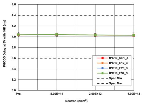
Figure 14. ISL70321SEH power-good delay with  $10k\Omega$  resistor ( $t_{PG_10}$ ) at  $V_{DD}$  = 3V following irradiation to each level. The error bars (if visible) represent the minimum and maximum measured values. The SMD limits are 3.6ms minimum and 4.4ms maximum.
