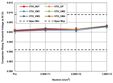
Figure 8. ISL70321SEH comparator rising threshold voltage ( $V_{TH}$ ) at  $V_{DD}$  = 3V following irradiation to each level. The error bars (if visible) represent the minimum and maximum measured values. The SMD limits are 0.591V minimum and 0.609V maximum.
