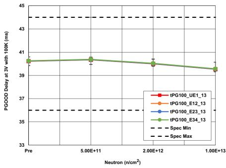
Figure 17. ISL70321SEH power-good delay with  $100k\Omega$  resistor ( $t_{PG_{100}}$ ) at  $V_{DD}$  = 13.2V following irradiation to each level. The error bars (if visible) represent the minimum and maximum measured values. The SMD limits are 36ms minimum and 44ms maximum.
