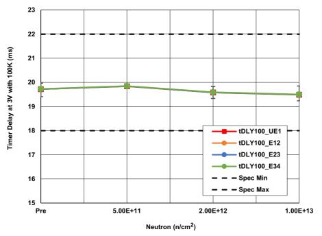
Figure 12. ISL70321SEH timer delay with 100k $\Omega$  resistor (t<sub>DLY\_100</sub>) at V<sub>DD</sub> = 3V following irradiation to each level. The error bars (if visible) represent the minimum and maximum measured values. The SMD limits are 18ms minimum and 22ms maximum.
