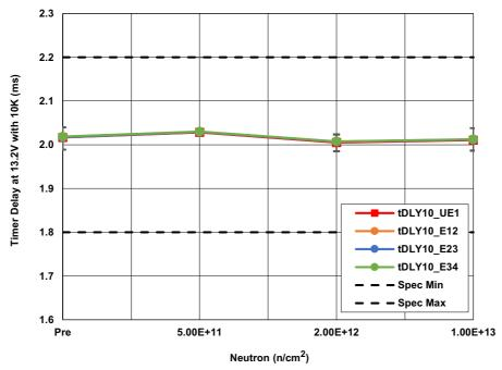
Figure 11. ISL70321SEH timer delay with  $10k\Omega$  resistor ( $t_{DLY_{10}}$ ) at  $V_{DD}$  = 13.2V following irradiation to each level. The error bars (if visible) represent the minimum and maximum measured values. The SMD limits are 1.8ms minimum and 2.2ms maximum.
