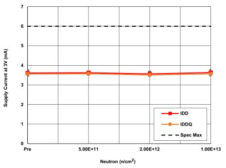
Figure 2. ISL70321SEH quiescent ( $I_{DDQ}$ ) and operating ( $I_{DD}$ ) supply current at  $V_{DD}$  = 3V following irradiation to each level. The error bars (if visible) represent the minimum and maximum measured values. The SMD limit is 6mA maximum.
