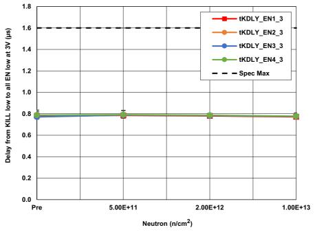
Figure 19. ISL70321SEH delay from KILL low to EN1 - EN4 Low ( $t_{KDLY}$ ) at  $V_{DD}$  = 3V irradiation to each level. The error bars (if visible) represent the minimum and maximum measured values. The SMD limit is 1.6µs maximum.
