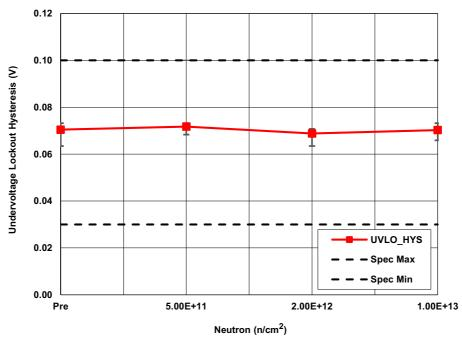
Figure 5. ISL70321SEH undervoltage lockout hysteresis (UVLO\_HYS) voltage following irradiation to each level. The error bars (if visible) represent the minimum and maximum measured values. The SMD limits are 0.03V minimum and 0.1V maximum.
