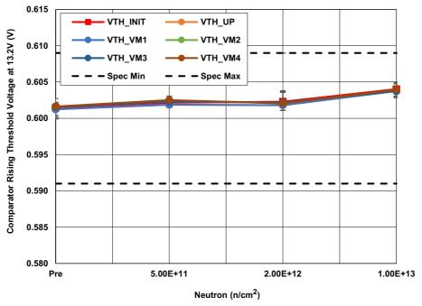
Figure 9. ISL70321SEH comparator rising threshold voltage ( $V_{TH}$ ) at  $V_{DD}$  = 13.2V following irradiation to each level. The error bars (if visible) represent the minimum and maximum measured values. The SMD limits are 0.591V minimum and 0.609V maximum.
