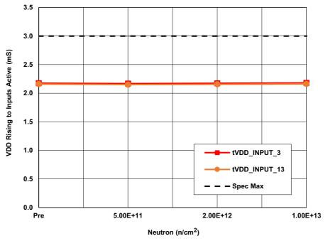
Figure 6. ISL70321SEH time from  $V_{DD}$  rising to inputs active ( $t_{VDD_INPUT}$ ) at  $V_{DD}$  = 3V and 13.2V following irradiation to each level. The error bars (if visible) represent the minimum and maximum measured values. The SMD limit is 3ms maximum.
