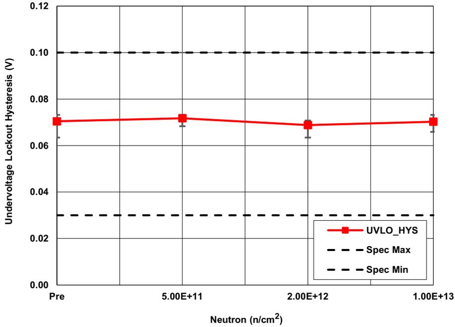
Figure 5. ISL70321SEH undervoltage lockout hysteresis (UVLO\_HYS) voltage following irradiation to each level. The error bars (if visible) represent the minimum and maximum measured values. The SMD limits are 0.03V minimum and 0.1V maximum.
