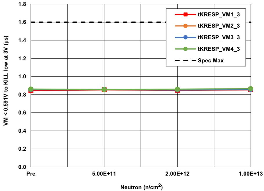
Figure 21. ISL70321SEH delay from VM < 0.591V to KILL Low ( $t_{KRESP}$ ) at  $V_{DD} = 3V$  irradiation to each level. The error bars (if visible) represent the minimum and maximum measured values. The SMD limit is 1.6µs maximum.
