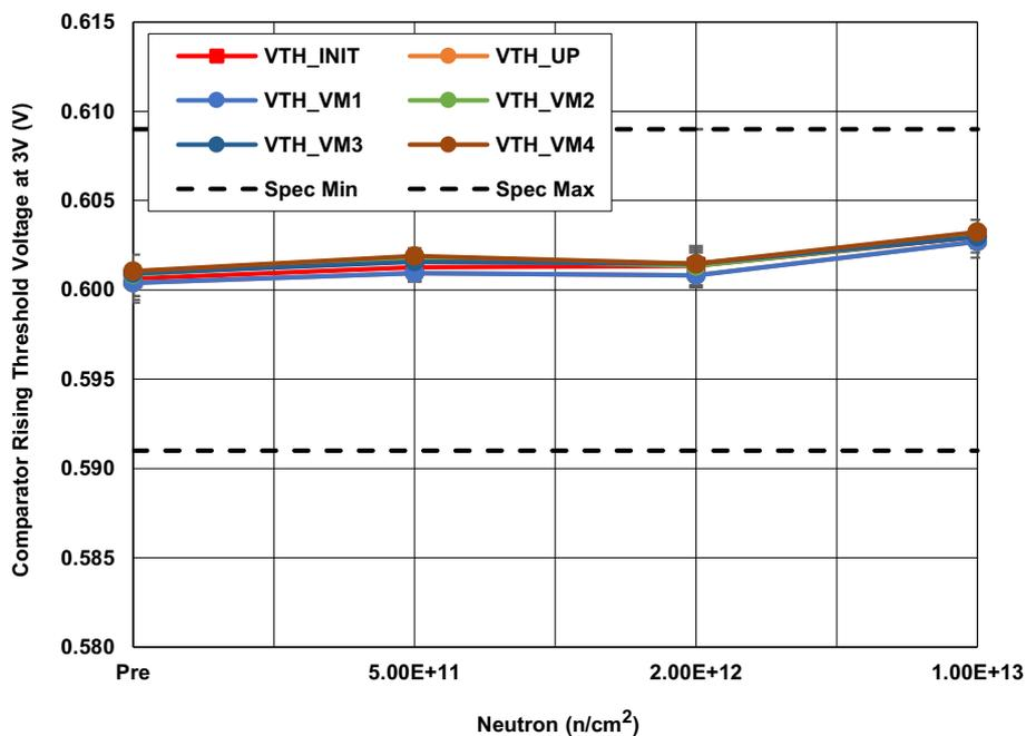
Figure 8. ISL70321SEH comparator rising threshold voltage ( $V_{TH}$ ) at  $V_{DD} = 3V$  following irradiation to each level. The error bars (if visible) represent the minimum and maximum measured values. The SMD limits are  $0.591V$  minimum and  $0.609V$  maximum.
