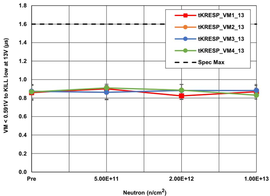
Figure 22. ISL70321SEH delay from VM < 0.591V to KILL Low ( $t_{KRESP}$ ) at  $V_{DD} = 13.2V$  irradiation to each level. The error bars (if visible) represent the minimum and maximum measured values. The SMD limit is 1.6µs maximum.
