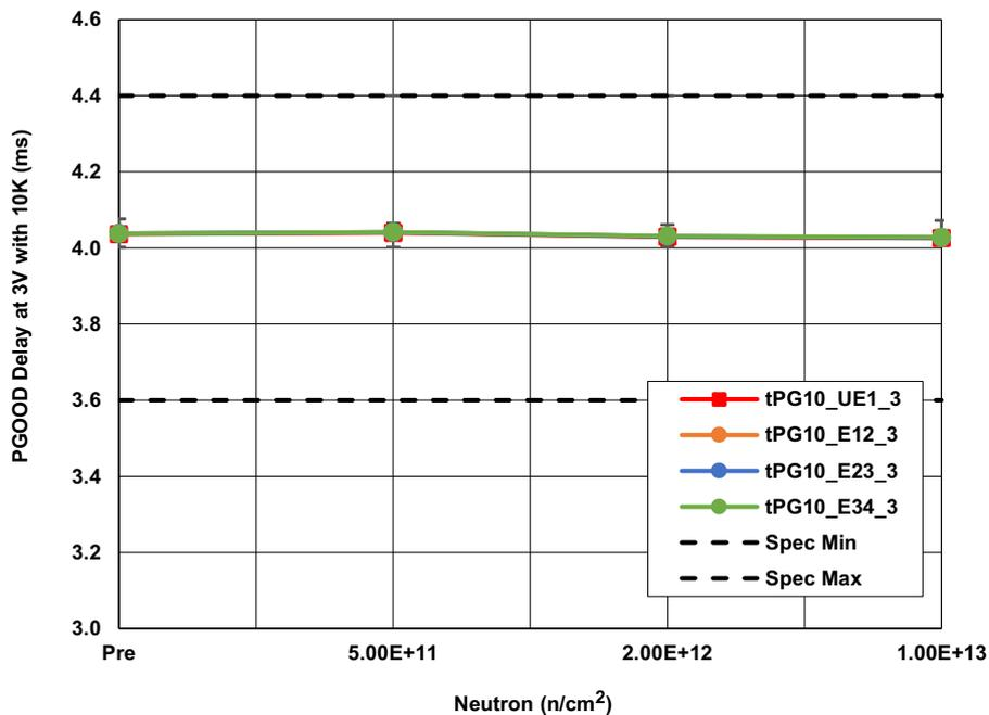
Figure 14. ISL70321SEH power-good delay with 10kΩ resistor ( $t_{PG\_10}$ ) at  $V_{DD} = 3V$  following irradiation to each level. The error bars (if visible) represent the minimum and maximum measured values. The SMD limits are 3.6ms minimum and 4.4ms maximum.
