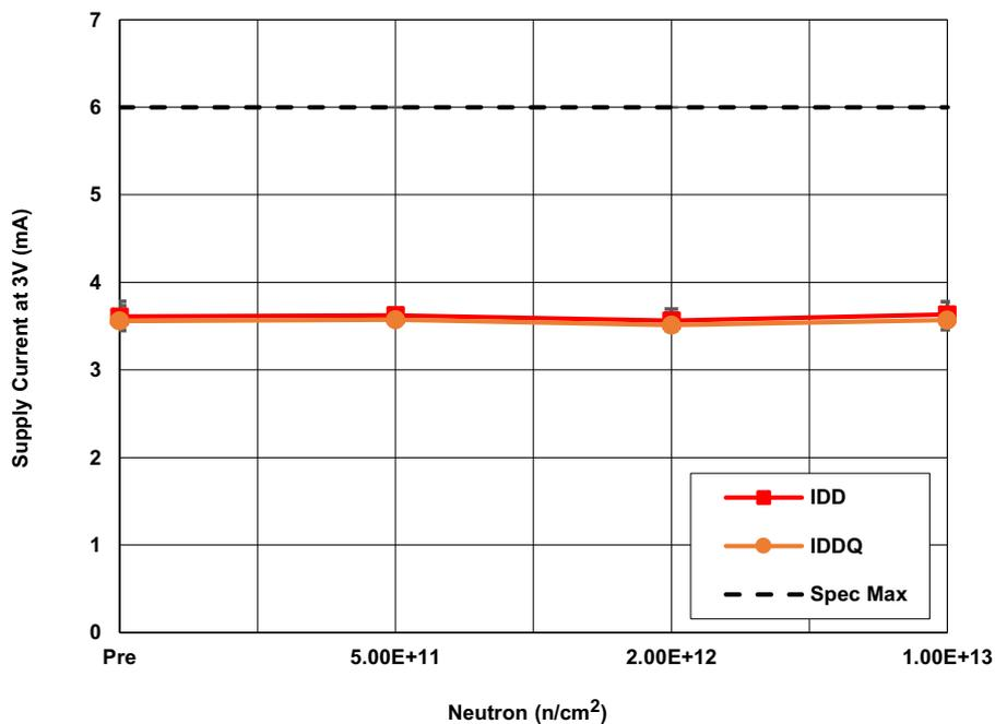
Figure 2. ISL70321SEH quiescent (I<sub>DDQ</sub>) and operating (I<sub>DD</sub>) supply current at V<sub>DD</sub> = 3V following irradiation to each level. The error bars (if visible) represent the minimum and maximum measured values. The SMD limit is 6mA maximum.
