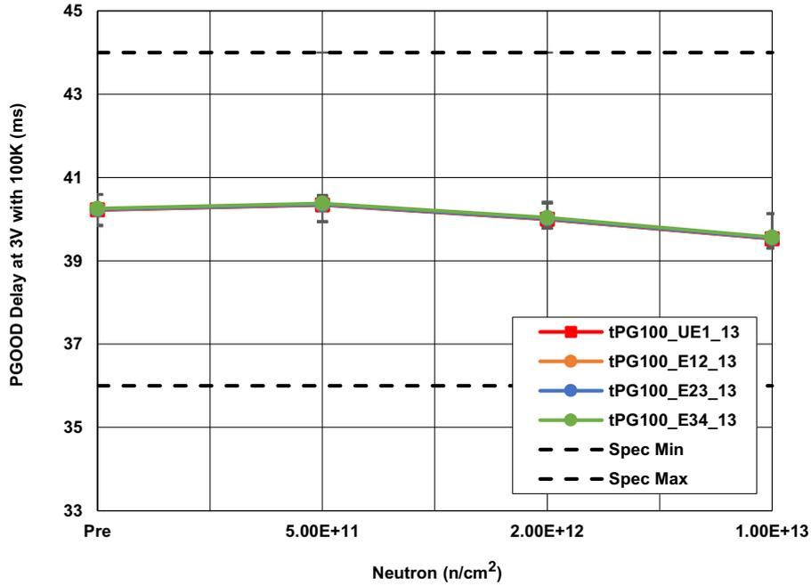
Figure 17. ISL70321SEH power-good delay with 100kΩ resistor ( $t_{PG\_100}$ ) at  $V_{DD} = 13.2V$  following irradiation to each level. The error bars (if visible) represent the minimum and maximum measured values. The SMD limits are 36ms minimum and 44ms maximum.
