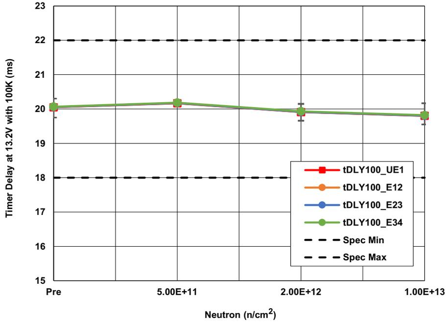
Figure 13. ISL70321SEH timer delay with 100kΩ resistor ( $t_{DLY\_100}$ ) at  $V_{DD} = 13.2V$  following irradiation to each level. The error bars (if visible) represent the minimum and maximum measured values. The SMD limits are 18ms minimum and 22ms maximum.
