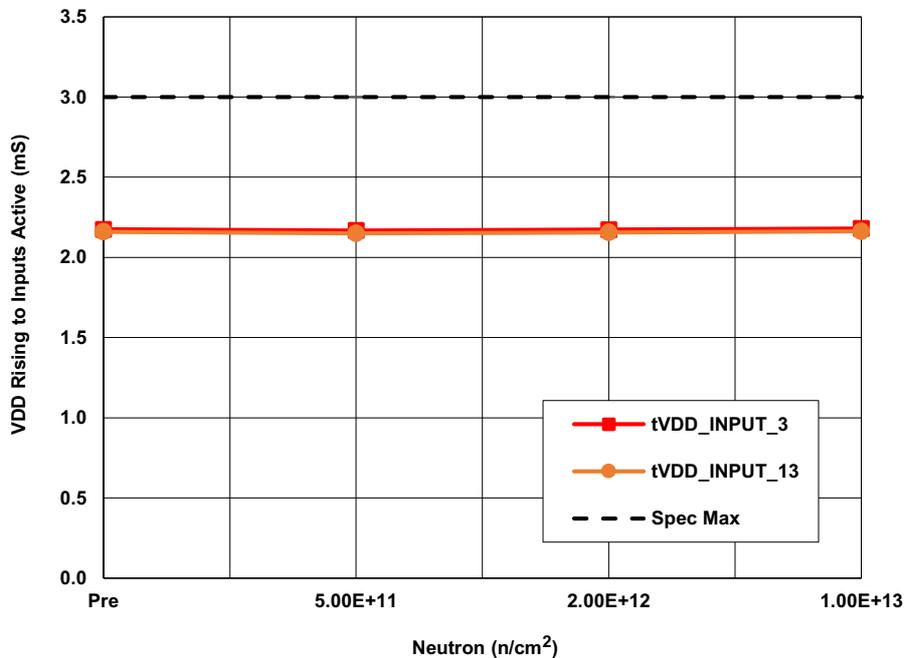
Figure 6. ISL70321SEH time from V<sub>DD</sub> rising to inputs active (t<sub>VDD\_INPUT</sub>) at V<sub>DD</sub> = 3V and 13.2V following irradiation to each level. The error bars (if visible) represent the minimum and maximum measured values. The SMD limit is 3ms maximum.
