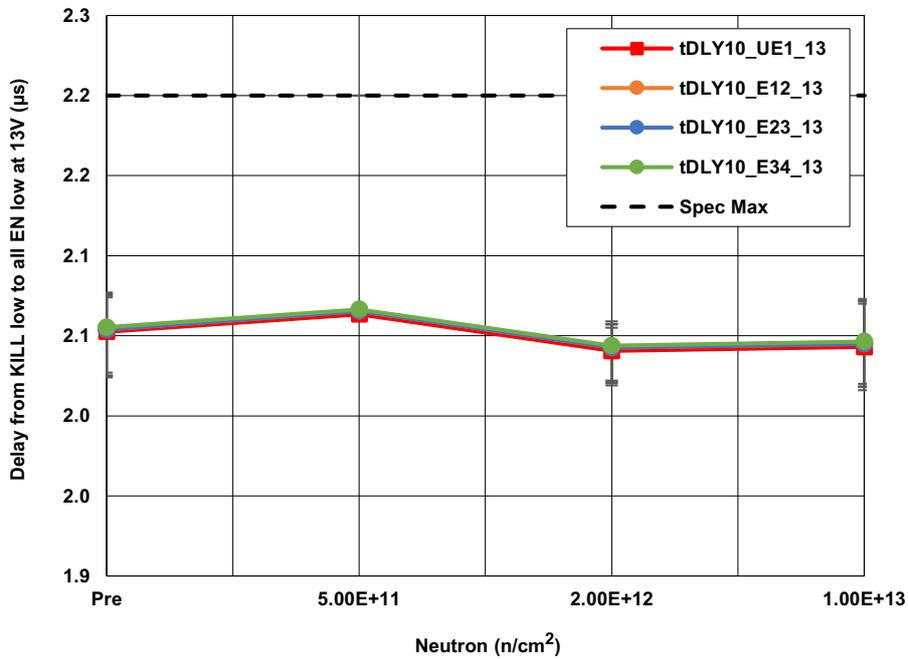
Figure 20. ISL70321SEH delay from KILL low to EN1 - EN4 Low ( $t_{KDLY}$ ) at  $V_{DD} = 13.2V$  irradiation to each level. The error bars (if visible) represent the minimum and maximum measured values. The SMD limit is 2.2µs maximum.
