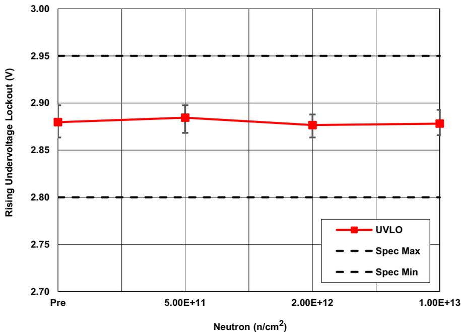
Figure 4. ISL70321SEH rising undervoltage lockout (UVLO) voltage following irradiation to each level. The error bars (if visible) represent the minimum and maximum measured values. The SMD limits are 2.80V minimum and 2.95V maximum.
