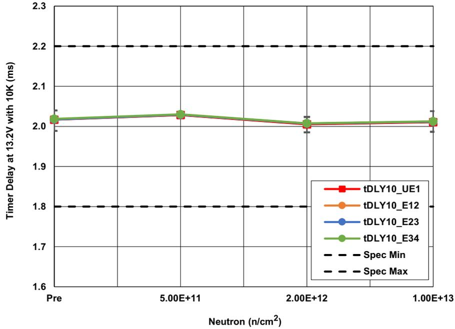
Figure 11. ISL70321SEH timer delay with 10kΩ resistor ( $t_{DLY\_10}$ ) at  $V_{DD} = 13.2V$  following irradiation to each level. The error bars (if visible) represent the minimum and maximum measured values. The SMD limits are 1.8ms minimum and 2.2ms maximum.
