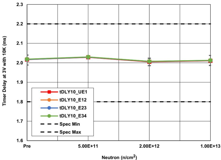
Figure 10. ISL70321SEH timer delay with 10KΩ resistor ( $t_{DLY\_10}$ ) at  $V_{DD} = 3V$  following irradiation to each level. The error bars (if visible) represent the minimum and maximum measured values. The SMD limits are 1.8ms minimum and 2.2ms maximum.
