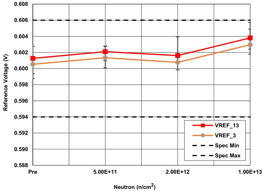
Figure 7. ISL70321SEH reference voltage ( $V_{REF}$ ) at  $V_{DD} = 3V$  and  $13.2V$  following irradiation to each level. The error bars (if visible) represent the minimum and maximum measured values. The SMD limits are  $0.594V$  minimum and  $0.606V$  maximum.
