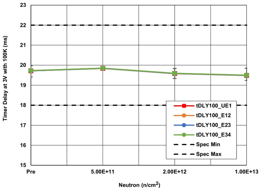
Figure 12. ISL70321SEH timer delay with 100kΩ resistor ( $t_{DLY\_100}$ ) at  $V_{DD} = 3V$  following irradiation to each level. The error bars (if visible) represent the minimum and maximum measured values. The SMD limits are 18ms minimum and 22ms maximum.
