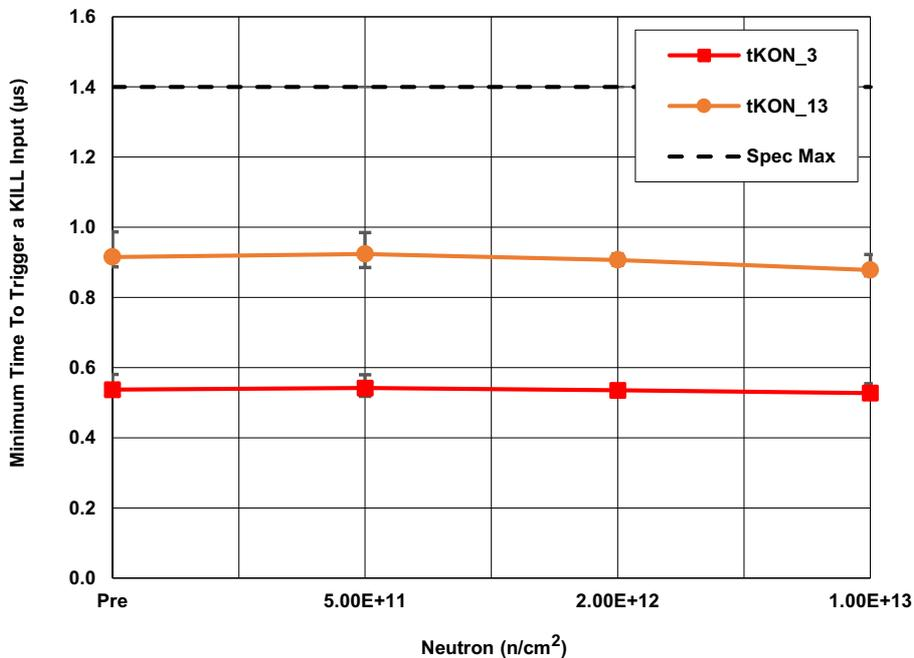
Figure 18. ISL70321SEH minimum time to trigger a KILL input ( $t_{KON}$ ) at  $V_{DD} = 3V$  and  $13.2V$  following irradiation to each level. The error bars (if visible) represent the minimum and maximum measured values. The SMD limit is 1.4µs maximum.
