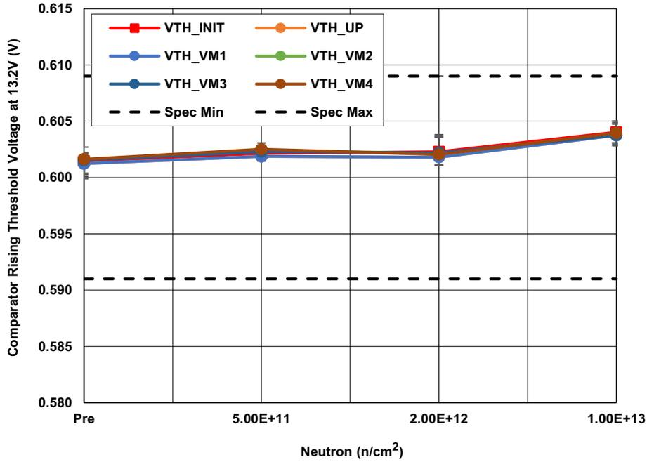
Figure 9. ISL70321SEH comparator rising threshold voltage ( $V_{TH}$ ) at  $V_{DD} = 13.2V$  following irradiation to each level. The error bars (if visible) represent the minimum and maximum measured values. The SMD limits are 0.591V minimum and 0.609V maximum.
