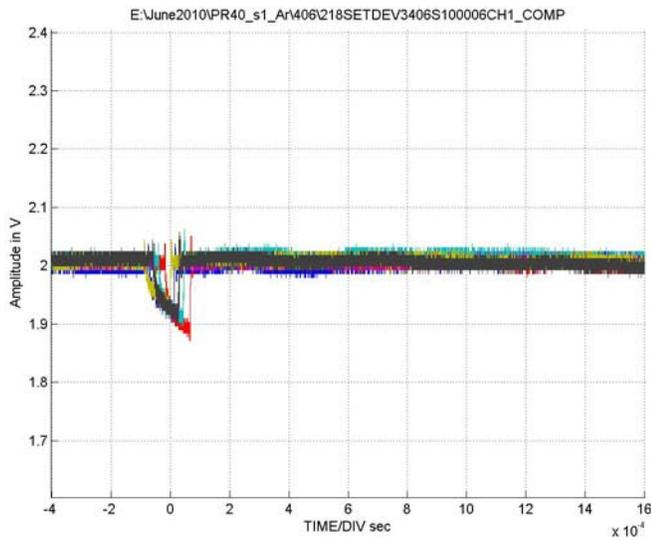
**FIGURE 15. TYPICAL CAPTURE AT  $V_S = \pm 18V$ , CHANNEL A, LET = 8.5MeV/mg/cm<sup>2</sup>, RUN 406**
