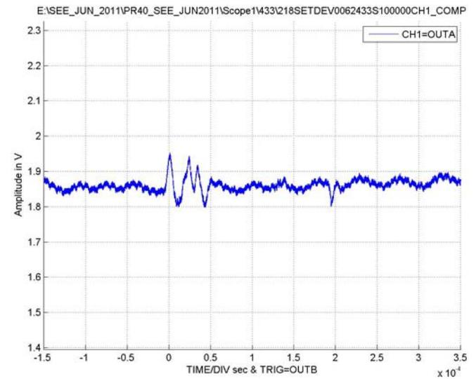
**FIGURE 10. TYPICAL CAPTURE AT  $V_S = \pm 18V$ , CHANNEL A, LET =  $2.7MeV/mg/cm^2$ , RUN 433**
