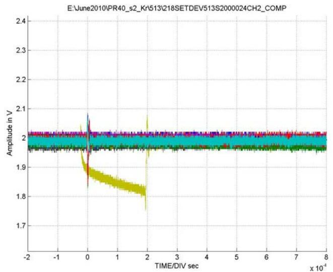
**FIGURE 26. TYPICAL CAPTURE AT  $V_S = \pm 4.5V$ , CHANNEL B, LET = 56MeV/mg/cm<sup>2</sup>, RUN 513**
