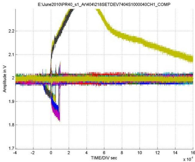
**FIGURE 19. TYPICAL CAPTURE AT  $V_S = \pm 18V$ , CHANNEL A, LET = 17MeV/mg/cm<sup>2</sup>, RUN 404**
