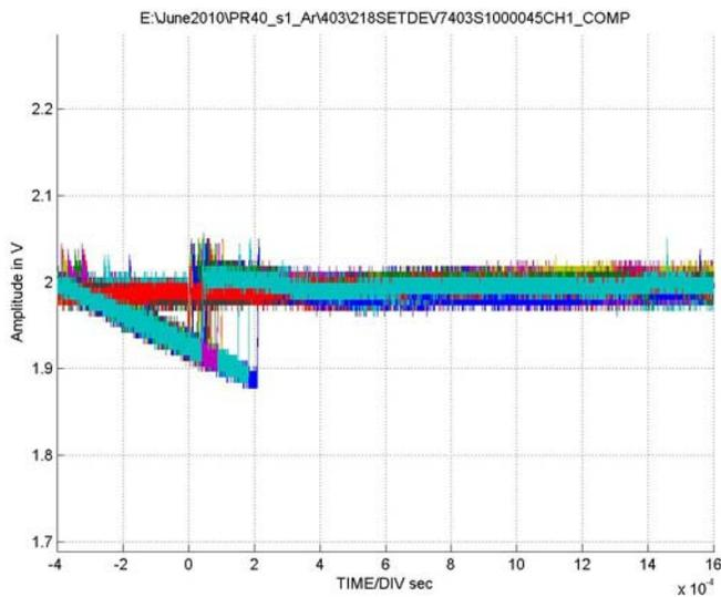
**FIGURE 17. TYPICAL CAPTURE AT  $V_S = \pm 4.5V$ , CHANNEL A, LET = 17MeV/mg/cm<sup>2</sup>, RUN 403**
