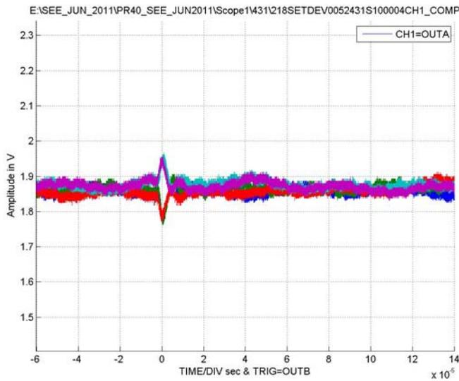
**FIGURE 11. TYPICAL CAPTURE AT  $V_S = \pm 18V$ , CHANNEL A, LET = 5.6MeV/mg/cm<sup>2</sup>, RUN 431**
