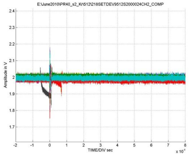
**FIGURE 24. TYPICAL CAPTURE AT  $V_S = \pm 18V$ , CHANNEL B, LET = 28MeV/mg/cm<sup>2</sup>, RUN 512**
