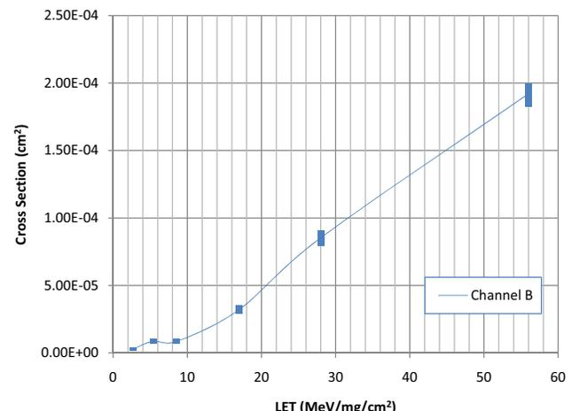
FIGURE 6. CHANNEL B CROSS SECTION VS. LET FOR  $V_S = \pm 18V$  WITH 90% CONFIDENCE LEVEL INTERVAL BARS
