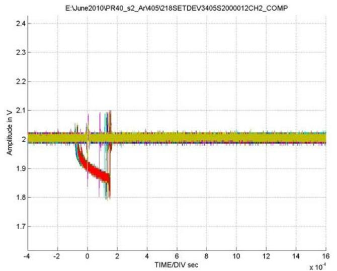
**FIGURE 14. TYPICAL CAPTURE AT  $V_S = \pm 4.5V$ , CHANNEL B, LET = 8.5MeV/mg/cm<sup>2</sup>, RUN 405**
