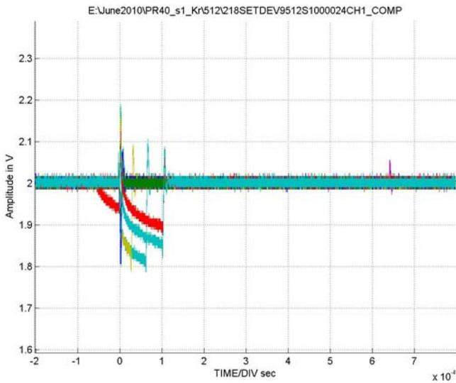
**FIGURE 23. TYPICAL CAPTURE AT  $V_S = \pm 18V$ , CHANNEL A, LET = 28MeV/mg/cm<sup>2</sup>, RUN 512**
