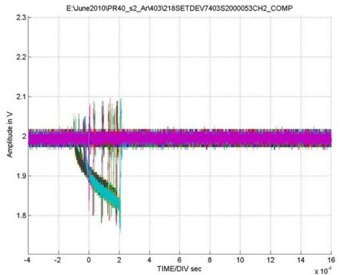
**FIGURE 18. TYPICAL CAPTURE AT  $V_S = \pm 4.5V$ , CHANNEL B, LET = 17MeV/mg/cm<sup>2</sup>, RUN 403**
