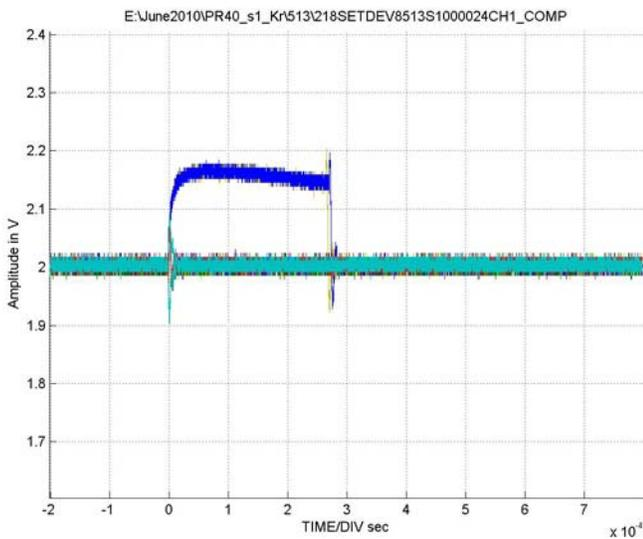
**FIGURE 25. TYPICAL CAPTURE AT  $V_S = \pm 4.5V$ , CHANNEL A, LET = 56MeV/mg/cm<sup>2</sup>, RUN 513**
