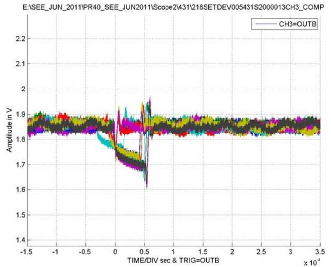
**FIGURE 12. TYPICAL CAPTURE AT  $V_S = \pm 18V$ , CHANNEL B, LET = 5.6MeV/mg/cm<sup>2</sup>, RUN 432**
