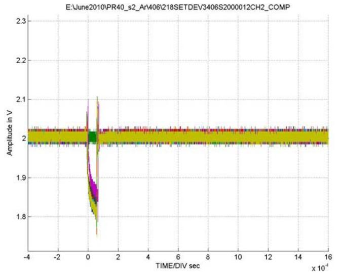
**FIGURE 16. TYPICAL CAPTURE AT  $V_S = \pm 18V$ , CHANNEL B, LET = 8.5MeV/mg/cm<sup>2</sup>, RUN 406**
