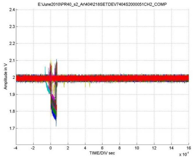
**FIGURE 20. TYPICAL CAPTURE AT  $V_S = \pm 18V$ , CHANNEL B, LET = 17MeV/mg/cm<sup>2</sup>, RUN 404**
