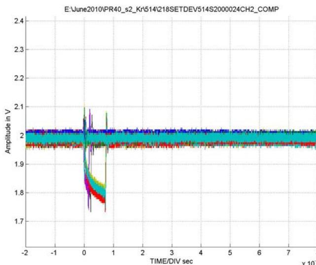
FIGURE 28. TYPICAL CAPTURE AT  $V_S = \pm 18V$ , CHANNEL B, LET = 56MeV/mg/cm<sup>2</sup>, RUN 514
