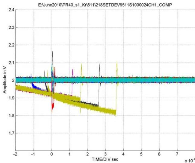
**FIGURE 21. TYPICAL CAPTURE AT  $V_S = \pm 4.5V$ , CHANNEL A, LET = 28MeV/mg/cm<sup>2</sup>, RUN 511**
