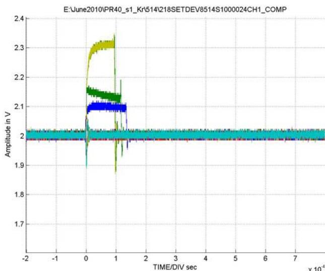
FIGURE 27. TYPICAL CAPTURE AT  $V_S = \pm 18V$ , CHANNEL A, LET = 56MeV/mg/cm<sup>2</sup>, RUN 514
