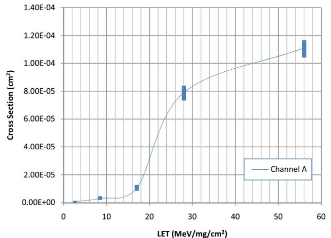
FIGURE 4. CHANNEL B CROSS SECTION VS. LET FOR  $V_S = \pm 4.5V$  WITH 90% CONFIDENCE LEVEL INTERVAL BARS
