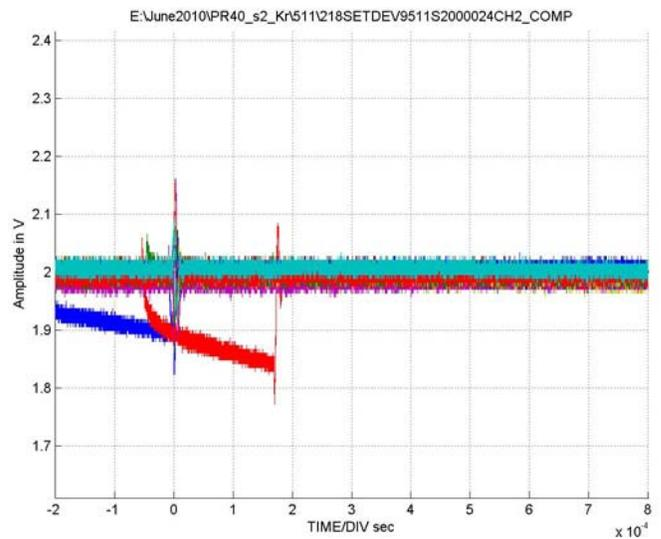
**FIGURE 22. TYPICAL CAPTURE AT  $V_S = \pm 4.5V$ , CHANNEL B, LET = 28MeV/mg/cm<sup>2</sup>, RUN 511**
