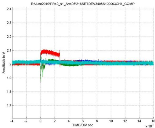
**FIGURE 13. TYPICAL CAPTURE AT  $V_S = \pm 4.5V$ , CHANNEL A, LET = 8.5MeV/mg/cm<sup>2</sup>, RUN 405**
