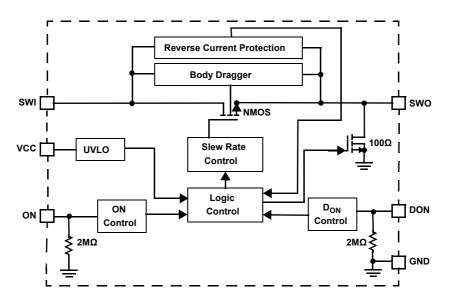
Figure 1. ISL70062SEH Block Diagram
