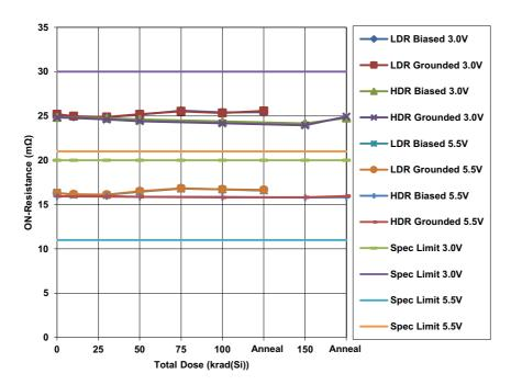
Figure 3. ISL70062SEH switch ON-resistance, 3.0V and 5.5V supply voltage,  $V_{SWI} = 1.0V$ , as a function of total dose irradiation at LDR and HDR for the biased and unbiased cases. The irradiations were followed by a high temperature biased anneal at 100°C for 168 hours. The LDR was 0.01rad(Si)/s and the HDR was 72rad(Si)/s. Sample sizes are given in Table 1. The post-irradiation SMD limits are 20m $\Omega$  to 30m $\Omega$  (3.0V supply) and 11m $\Omega$  to 21m $\Omega$  (5.5V supply).
