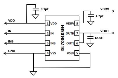
Figure 1. Schematic of the ISL70040SEH SEE testing circuit. Connectors indicated go to 20 foot cables connecting to the control room. C<sub>OUT</sub> and V<sub>DD</sub> varied depending on the test.
