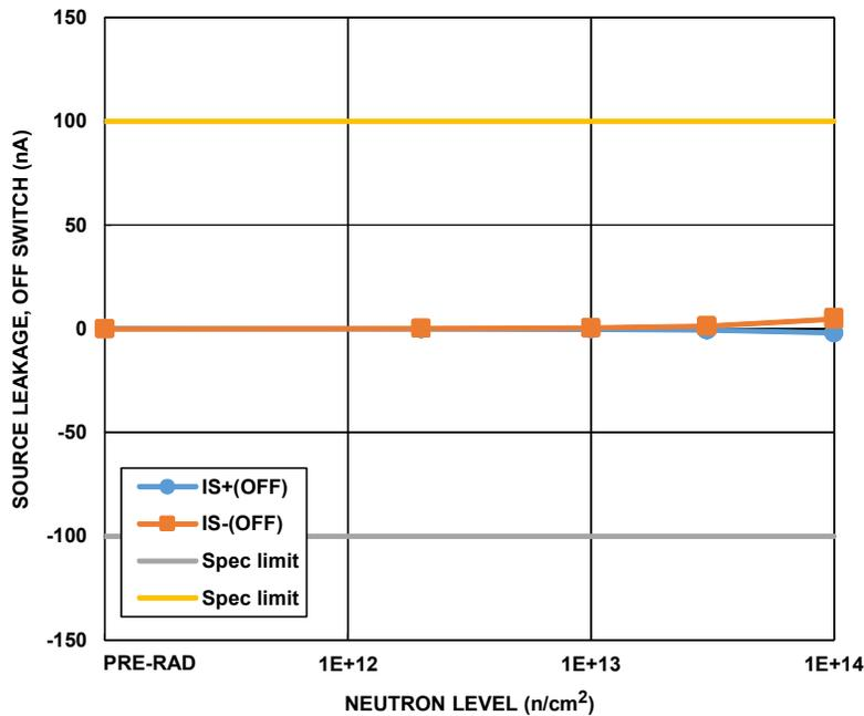
**FIGURE 5.** HS-303ARH leakage current into the source terminal of an OFF switch, Channel 1, as a function of 1MeV equivalent neutron irradiation at  $2 \times 10^{12} \text{ n/cm}^2$ ,  $1 \times 10^{13} \text{ n/cm}^2$ ,  $3 \times 10^{13} \text{ n/cm}^2$  and  $1 \times 10^{14} \text{ n/cm}^2$ . The plot shows the population median and minimum and maximum error bars at each datapoint. Sample size for each cell was 5. The post-total dose irradiation SMD limits are -100nA to 100nA.
