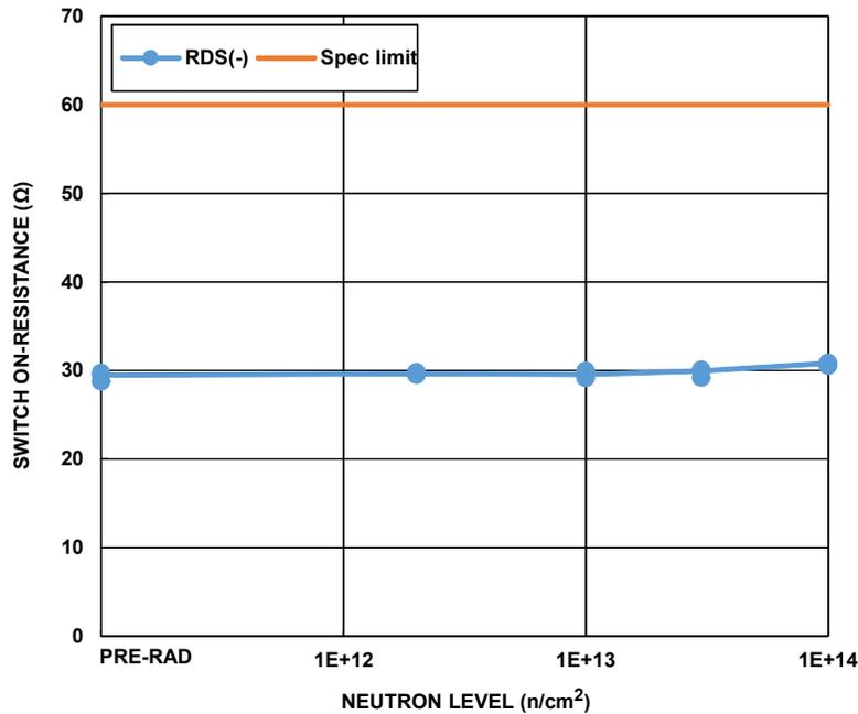
**FIGURE 4.** HS-303ARH switch ON-resistance, drain voltage -10V, as a function of 1MeV equivalent neutron irradiation at  $2 \times 10^{12} \text{ n/cm}^2$ ,  $1 \times 10^{13} \text{ n/cm}^2$ ,  $3 \times 10^{13} \text{ n/cm}^2$  and  $1 \times 10^{14} \text{ n/cm}^2$ . The plot shows the population median and minimum and maximum error bars at each datapoint. Sample size for each cell was 5. The post-total dose irradiation SMD limit is 60Ω maximum.
