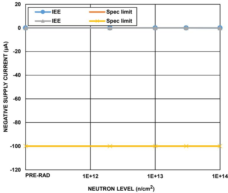
**FIGURE 2.** HS-303ARH negative supply current as a function of 1MeV equivalent neutron irradiation at  $2 \times 10^{12} \text{ n/cm}^2$ ,  $1 \times 10^{13} \text{ n/cm}^2$ ,  $3 \times 10^{13} \text{ n/cm}^2$  and  $1 \times 10^{14} \text{ n/cm}^2$ . The plot shows the population median and minimum and maximum error bars at each datapoint. Sample size for each cell was 5. The post-total dose irradiation SMD limit is  $-100 \mu\text{A}$  minimum.
