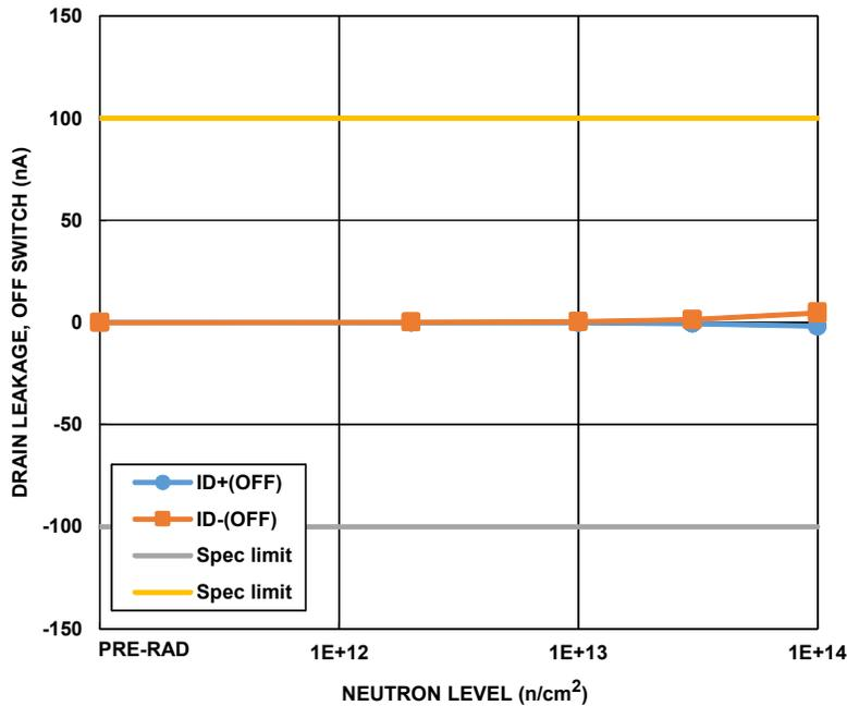
**FIGURE 6.** HS-303ARH leakage current into the drain terminal of an OFF switch, Channel 1, as a function of 1MeV equivalent neutron irradiation at  $2 \times 10^{12} \text{ n/cm}^2$ ,  $1 \times 10^{13} \text{ n/cm}^2$ ,  $3 \times 10^{13} \text{ n/cm}^2$  and  $1 \times 10^{14} \text{ n/cm}^2$ . The plot shows the population median and minimum and maximum error bars at each datapoint. Sample size for each cell was 5. The post-total dose irradiation SMD limits are -100nA to 100nA.
