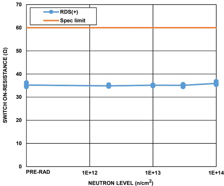
**FIGURE 3.** HS-303ARH switch ON-resistance, drain voltage +10V, as a function of 1MeV equivalent neutron irradiation at  $2 \times 10^{12} \text{ n/cm}^2$ ,  $1 \times 10^{13} \text{ n/cm}^2$ ,  $3 \times 10^{13} \text{ n/cm}^2$  and  $1 \times 10^{14} \text{ n/cm}^2$ . The plot shows the population median and minimum and maximum error bars at each datapoint. Sample size for each cell was 5. The post-total dose irradiation SMD limit is  $60 \Omega$  maximum.
