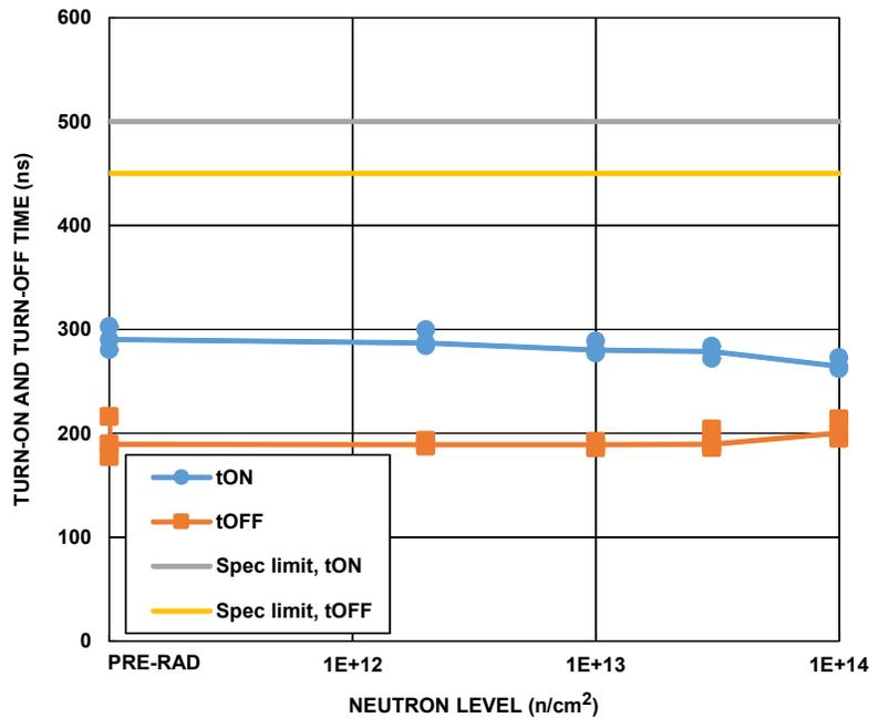
**FIGURE 10.** HS-303ARH switch turn-on and turn-off time as a function of 1MeV equivalent neutron irradiation at  $2 \times 10^{12} \text{ n/cm}^2$ ,  $1 \times 10^{13} \text{ n/cm}^2$ ,  $3 \times 10^{13} \text{ n/cm}^2$  and  $1 \times 10^{14} \text{ n/cm}^2$ . The plot shows the population median and minimum and maximum error bars at each datapoint. Sample size for each cell was 5. The post-total dose irradiation SMD limits are 500ns maximum (turn-on time) and 450ns maximum (turn-off time).
