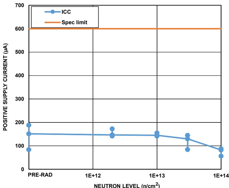
FIGURE 1. HS-303ARH positive supply current as a function of 1MeV equivalent neutron irradiation at 2x10<sup>12</sup>n/cm<sup>2</sup>, 1x10<sup>13</sup>n/cm<sup>2</sup>, 3x10<sup>13</sup>n/cm<sup>2</sup> and 1x10<sup>14</sup>n/cm<sup>2</sup>. The plot shows the population median and minimum and maximum error bars at each downpoint. Sample size for each cell was 5. The post-total dose irradiation SMD limit is 600µA maximum.
