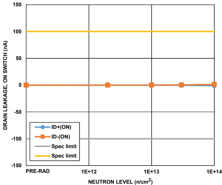
**FIGURE 7.** HS-303ARH leakage current into the drain terminal of an ON switch, Channel 1, as a function of 1MeV equivalent neutron irradiation at  $2 \times 10^{12} \text{ n/cm}^2$ ,  $1 \times 10^{13} \text{ n/cm}^2$ ,  $3 \times 10^{13} \text{ n/cm}^2$  and  $1 \times 10^{14} \text{ n/cm}^2$ . The plot shows the population median and minimum and maximum error bars at each datapoint. Sample size for each cell was 5. The post-total dose irradiation SMD limits are -100nA to 100nA.
