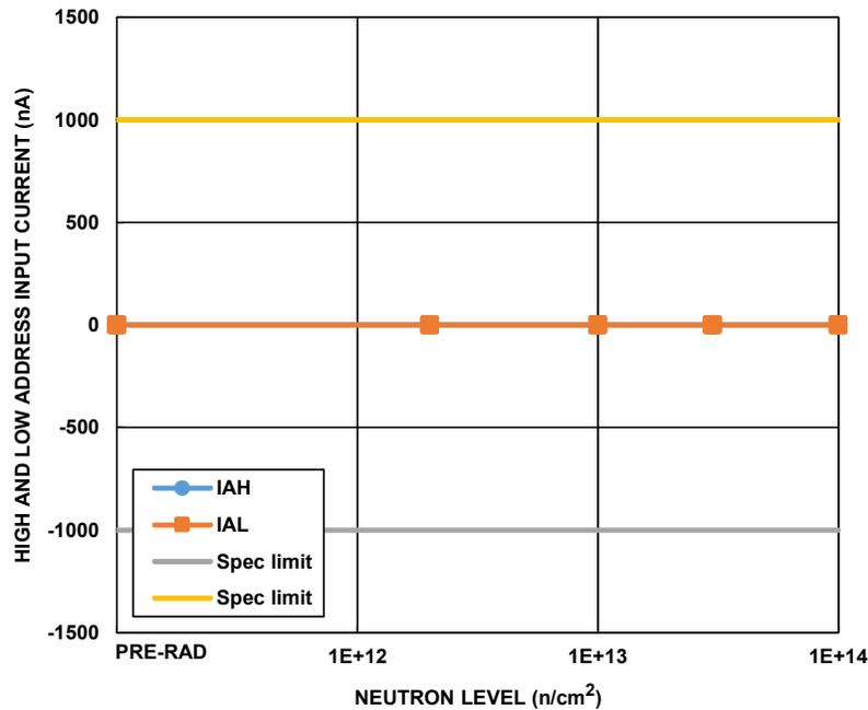
**FIGURE 8.** HS-303ARH HIGH and LOW address input current, address A1 as a function of 1MeV equivalent neutron irradiation at  $2 \times 10^{12} \text{ n/cm}^2$ ,  $1 \times 10^{13} \text{ n/cm}^2$ ,  $3 \times 10^{13} \text{ n/cm}^2$  and  $1 \times 10^{14} \text{ n/cm}^2$ . The plot shows the population median and minimum and maximum error bars at each datapoint. Sample size for each cell was 5. The post-total dose irradiation SMD limits are -1000nA to 1000nA.
