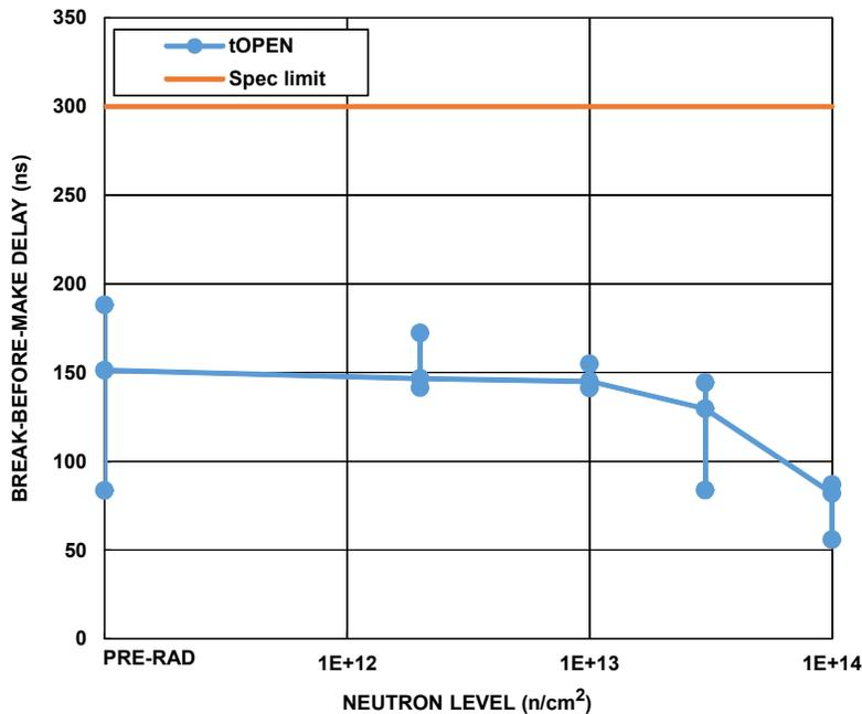
**FIGURE 9.** HS-303ARH break-before-make delay as a function of 1MeV equivalent neutron irradiation at  $2 \times 10^{12} \text{ n/cm}^2$ ,  $1 \times 10^{13} \text{ n/cm}^2$ ,  $3 \times 10^{13} \text{ n/cm}^2$  and  $1 \times 10^{14} \text{ n/cm}^2$ . The plot shows the population median and minimum and maximum error bars at each datapoint. Sample size for each cell was 5. The post-total dose irradiation SMD limits are 300ns maximum.
