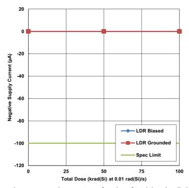
Figure 2. HS-303AEH negative power supply current as a function of total dose irradiation for the biased and unbiased cases. The dose rate was 0.01 rad(Si)/s and the sample size was 34 for each cell. The post-radiation SMD limit is -100 $\mu$ A minimum.
