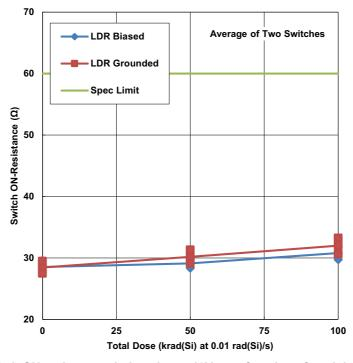
Figure 4. HS-303AEH switch ON-resistance, drain voltage -10V, as a function of total dose irradiation for the biased and unbiased cases. The dose rate was 0.01rad(Si)/s and the sample size was 34 for each cell. The post-radiation SMD limit is  $60\Omega$  maximum.
