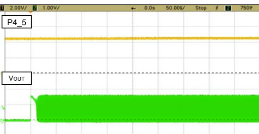
Oscillation start up waveform on recommendable circuit condition MODEL: CSTCE16M0V53-R0 with R5F21336TDFP(CM11=0)
