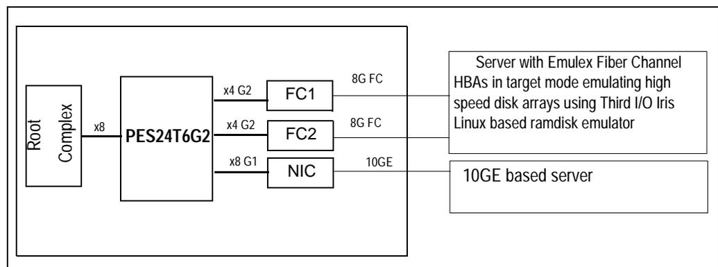
Figure 7 FC & GE Throughput Measurement Setup with the PES24T6G2 and two Fiber Ports
