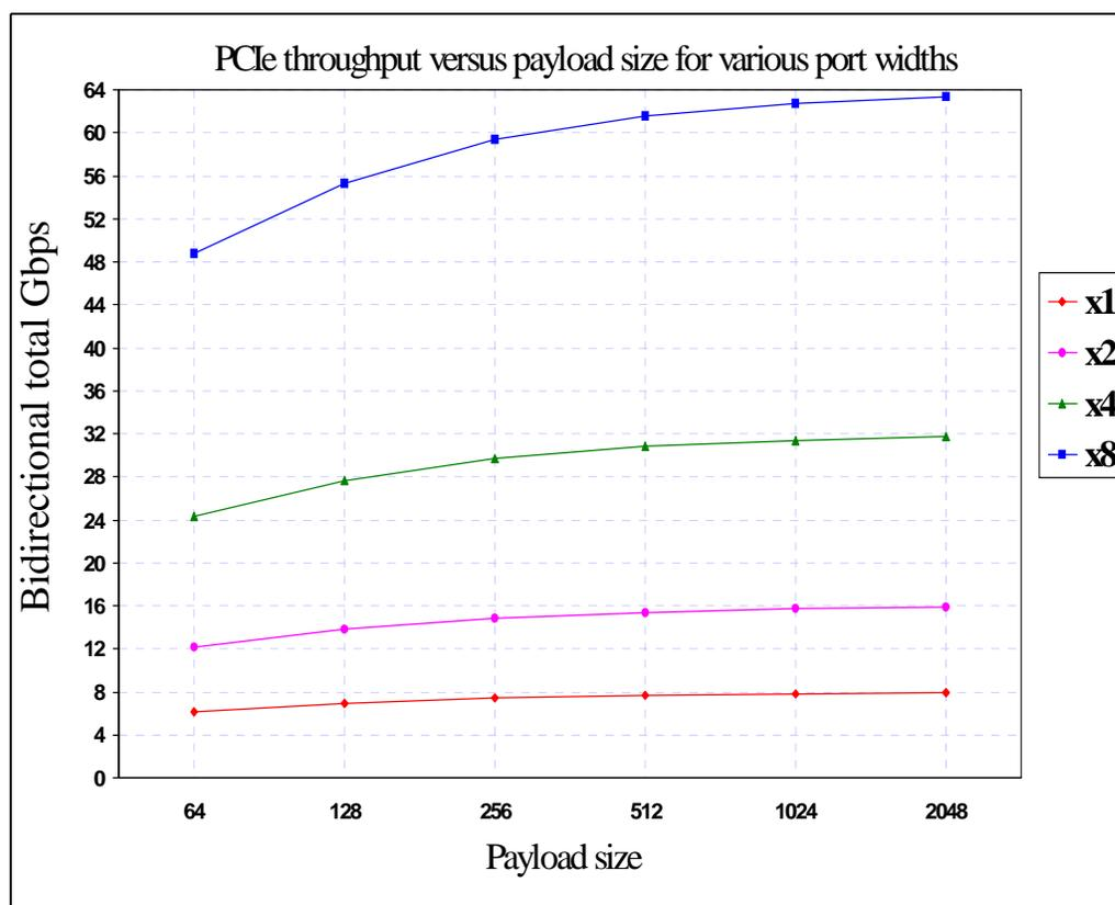
Figure 2 Effect of Framing Overhead on Link Efficiency
