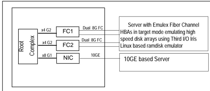
Figure 6 FC & GE Throughput Measurement without the PES24T6G2 and 4 Fiber Ports
