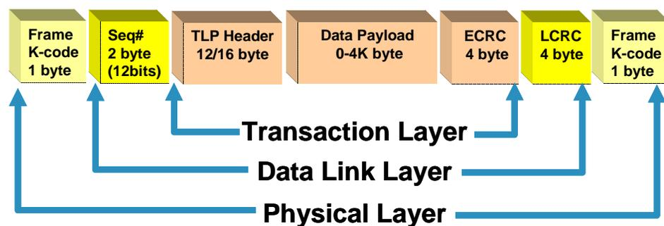
Figure 1 Framing Overhead in a Typical Transaction Packet
