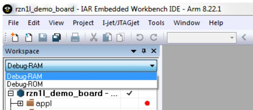
Figure 2-2: IAR Configurations RAM and ROM for RZ/N1L
