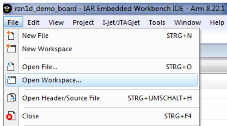
3. Go to the workspace folder and open it. In case the CPU board is used together with the extension board, please ensure to select the correct IAR-project.
