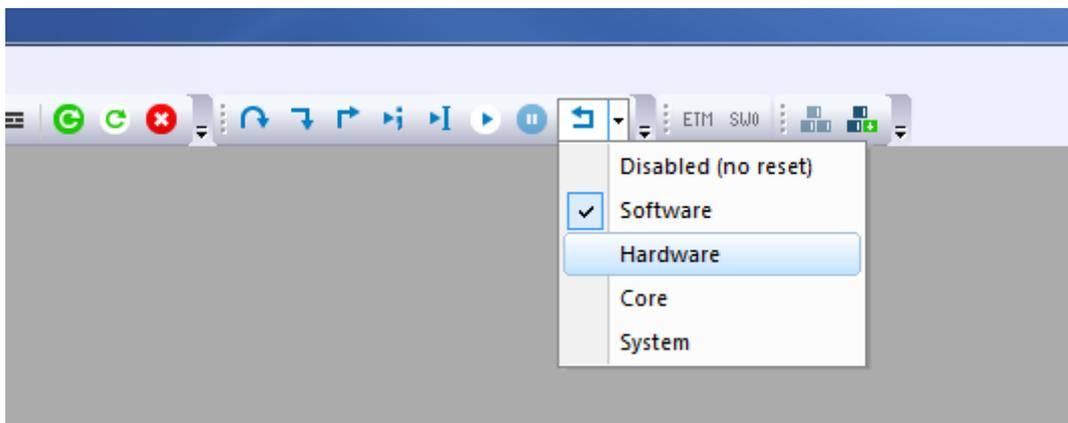
Figure 2-4: Changing Reset mode of RZ/N1L in Debug-ROM configuration
