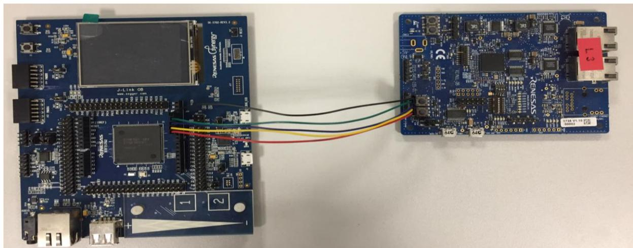
Figure 2-7: SPI connection of Synergy S7GS-SK (left) and RZ/N1L (right)
