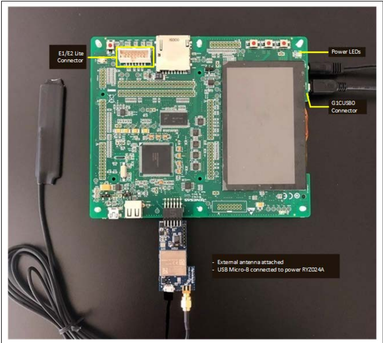
Figure 5. Connections to the RX65N-2MB Board After Flashing
