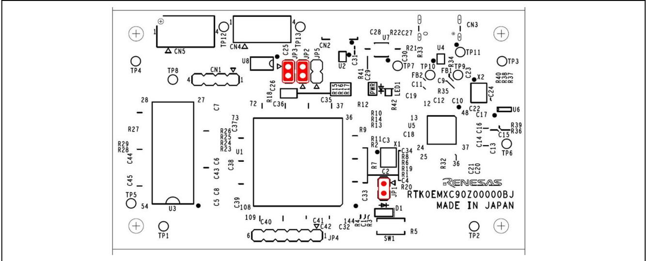
**Figure 4-3 Jumper pin setting of Communication Board**
