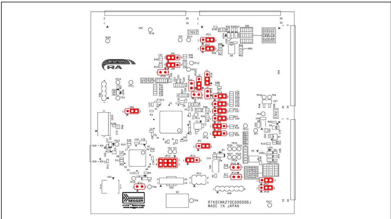
**Figure 4-2 Jumper pin setting of CPU Board**
