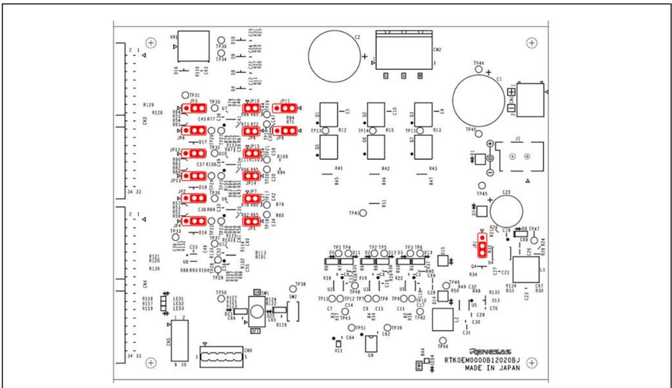
Figure 4-1 Jumper pin setting of Inverter Board
