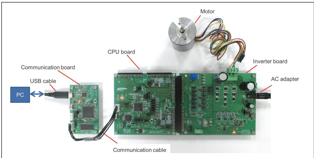
Figure 6-1 Hardware Configuration
