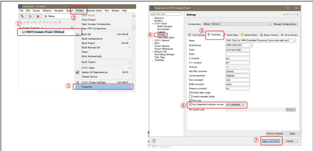
Figure 5-3 Toolchain configuration
