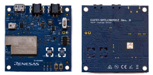
Figure 1: Top and back view of EU153-1 board
