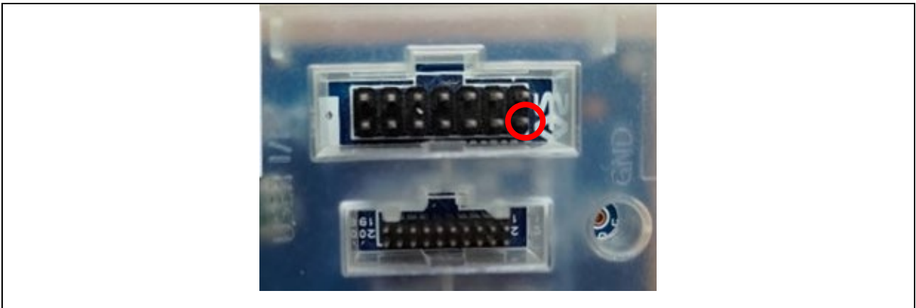
Figure 2.6 14pin connector GND pin position
