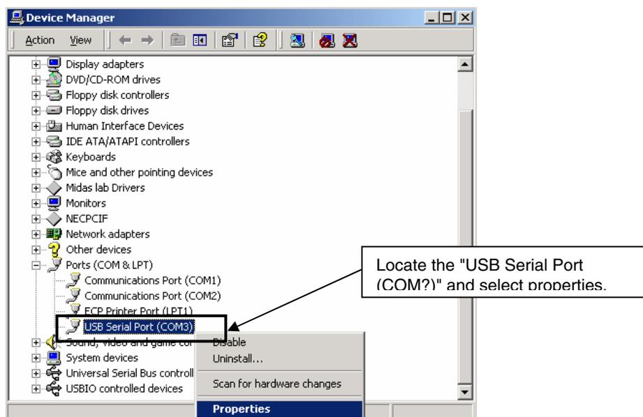
Figure 66: Configuration of COM port for IAR C-SPY debugger 1/4
