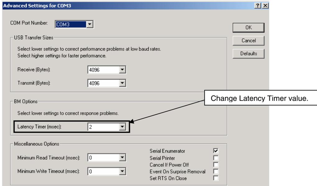
**Figure 69: Configuration of COM port for IAR C-SPY debugger 4/4**
