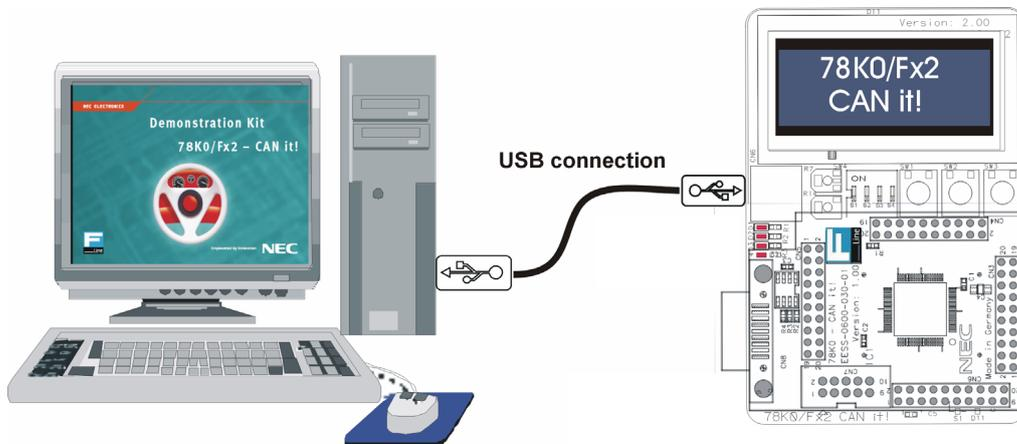
Figure 1: 78K0/Fx2 – CAN it! system configuration
