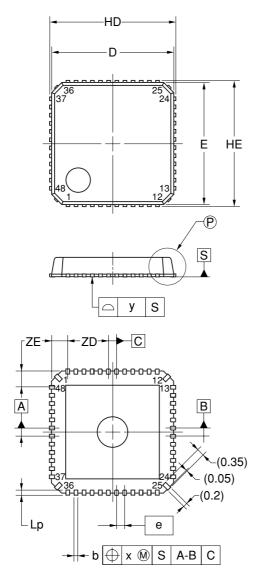
Although there are 4 terminals in the corner part of a package, these terminals are not designed for interconnection, but for manufacturing process of the package. Therefor do not intend to solder these 4 terminals, solderability of these 4 terminals are not guaranteed.
