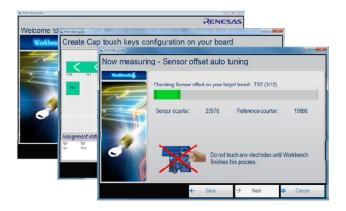
Sensitivity parameter automatic tuning screens. Even beginners can optimally tune sensitivity parameters and output source code simply by following along with the GUI style wizard interface.
